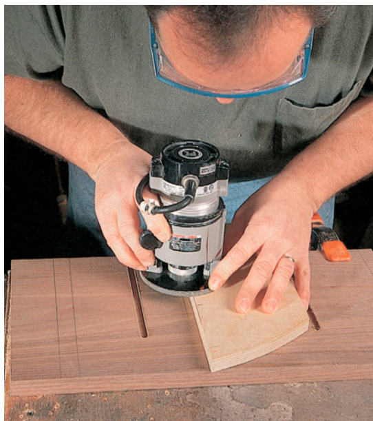
Four 1/4" dados are cut in each side to hold the drawer dividers. I like using a trim router for this step and also use a template guide with a straight bit and a piece of scrap wood as a straight edge.
