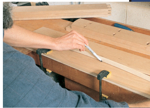
The graceful curves on the top and bottom brackets can be laid out with the aid of a helper by tracing along a bent strip of thin wood.
