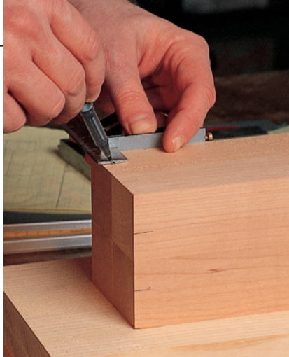
The diamond marked on the tops of the four legs will always allow you to recognize the inside and outside faces of the legs.
