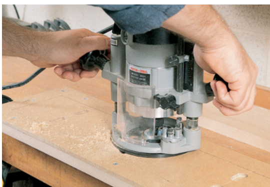
A plunge router plus a mortising jig equals precision mortises – something that's paramount when the mortises are through and the tenons are exposed.
