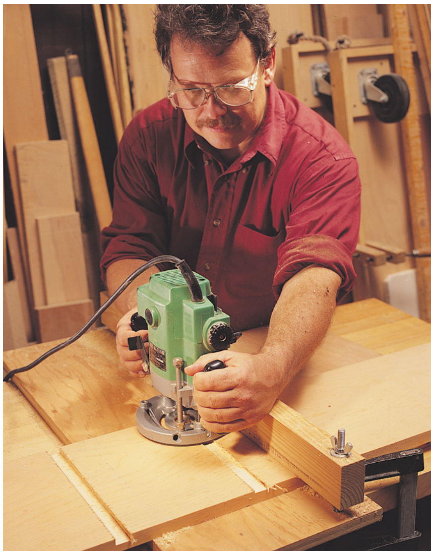
Cutting dados in long pieces of material is fast and easy with this simple jig.
