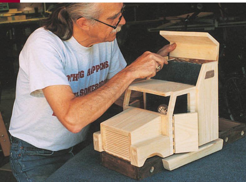
Prior to final installation, carpet the interior of the roof. I started the carpet where the top of the windshield meets the roof, about \frac{3}{4} " back from the leading edge.
