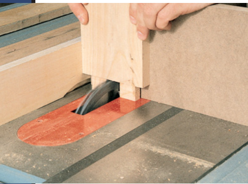
Clamping a tall support fence to your miter gauge will make cutting the twin tenons a safe and easy operation.
