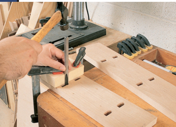
To guarantee the mortise corners end up perfectly vertical, clamp a scrap of wood flush with the edge of the mortise to guide the chisel.
