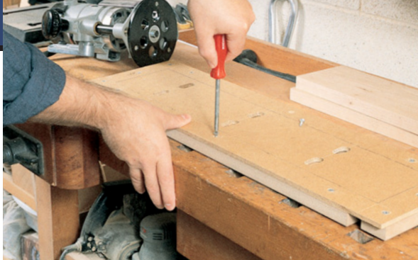
Cleats screwed around the perimeter of the mortising jig capture a side piece for routing the mortises.
