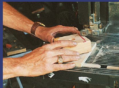
Then it's a simple matter of slowly rotating the stock to create a tire that needs just a little sanding.
