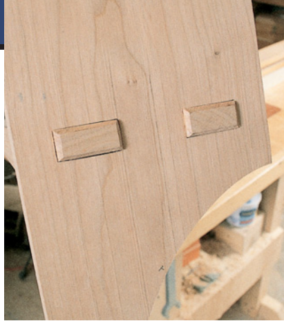
A friction fit of the tenons in the mortises is what you're looking for. You should feel just a slight resistance as you slide the pieces together.
