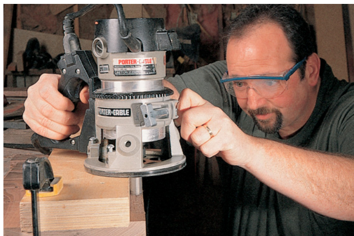
I switched bits and routers then cut a dado for the bottom in each side and a stopped rabbet on the back edge of each side to hold the 5/8" back boards in place.
