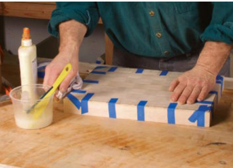
Begin veneering at the top. Liberal amounts of blue tape hold a veneer sheet securely in place on the top of the carcass.
