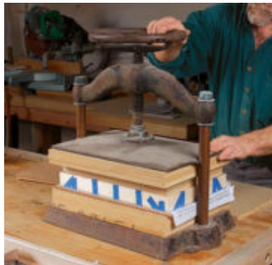
A box-sized caul. The top is clamped in an antique book press while the glue dries. A caul, made of layers of medium-density fiberboard (MDF) with cork padding on one face, provides even pressure. If you don't happen to own an antique book press, a pair of cauls and lots of clamps will do nicely.
