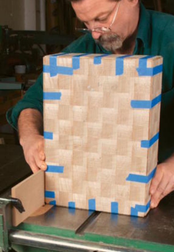
Grooves for binding. With top and bottom sections taped together temporarily, Janofsky cuts a shallow rabbet into each corner to hold the binding—thin strips of white oak.
