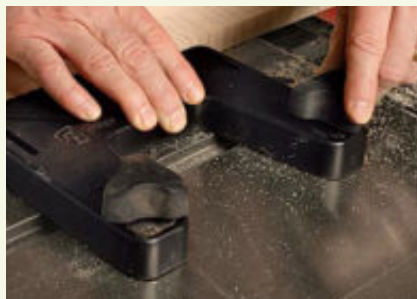
Magnetic attraction. The magnets in the Magswitch featherboard are activated by turning two knobs.
