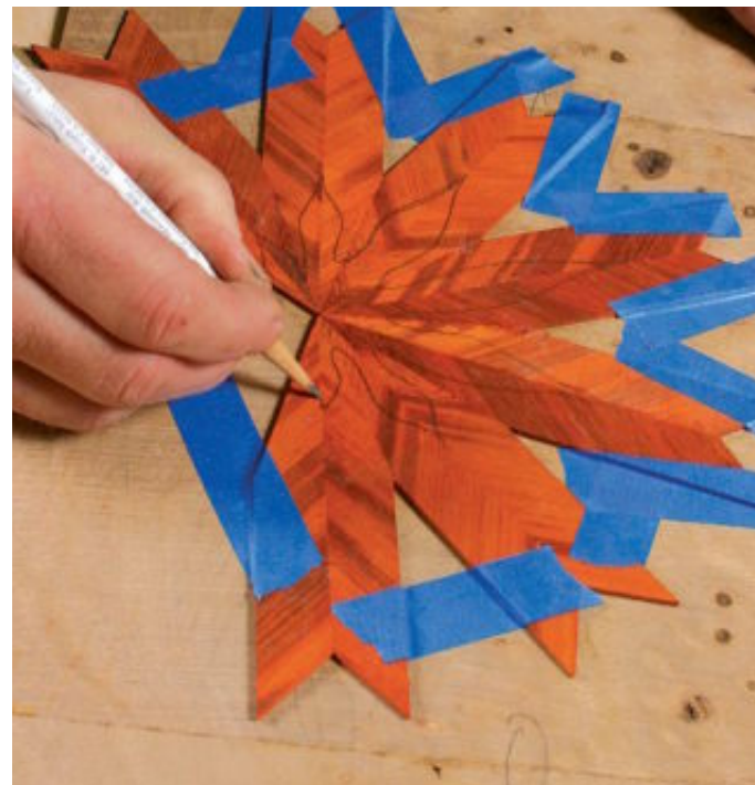
Position a blank and draw the shape. Tape the blank on the background veneer, then outline the leaf shape. You can draw freehand or trace a pattern, but let the shapes and sizes vary.
