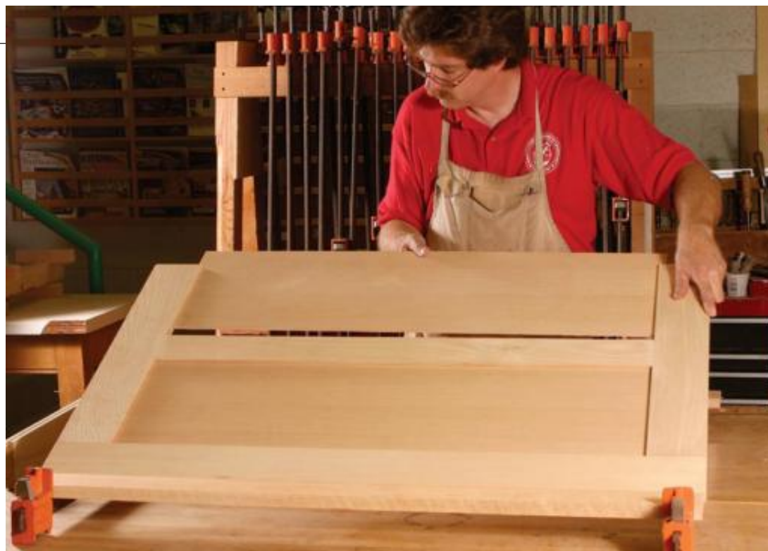
Assemble the back. The \frac{1}{2} -in.-thick plywood is rabbeted on the back side, ensuring a good fit in the grooves. Check carefully once the clamps are on to make sure the assembly is flat, tapping the components into place with a deadblow hammer, if needed, as you tighten the clamps.
