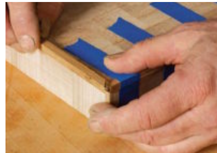
Top and bottom next. Rabbets are cut in the top and bottom for mitered pieces of binding. These pieces are cut slightly over-size, then planed flush.
