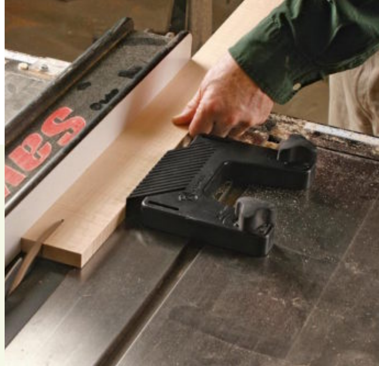
Safety where you need it. A featherboard helps keep the board snug to the fence at the start of the cut, where you have the least amount of control.
