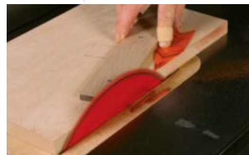
Point the ends. A simple 18° jig that rides in a miter slot on the tablesaw is used to sharpen the point of each chevron. Use a fine-tooth laminate blade to keep the cuts as clean as possible.
