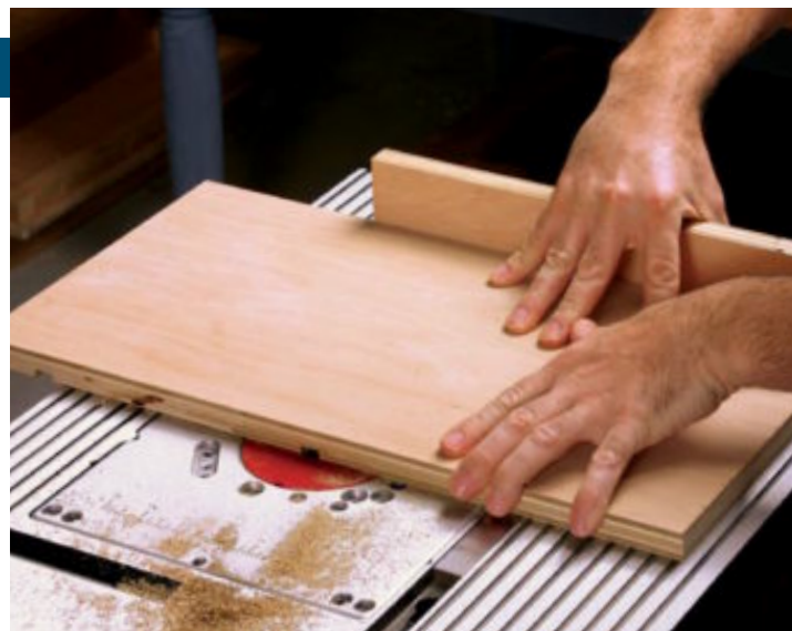
Remove the fence for interior dado cuts. A miter gauge with an attached fence keeps the cut straight.
