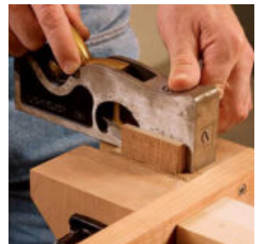
Tame your tenons. A shoulder plane can be used on its side (left) to trim a tenon’s cheeks. Used vertically (right), it can trim and square the tenon shoulders.
