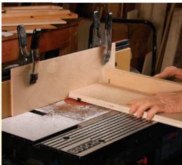
Router fence keeps dado cuts straight. For dadoes that are near the edge of a workpiece, use the fence to guide a clean and straight cut.
