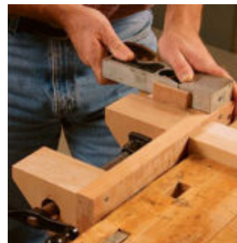
Tame your tenons. A shoulder plane can be used on its side (left) to trim a tenon’s cheeks. Used vertically (right), it can trim and square the tenon shoulders.
