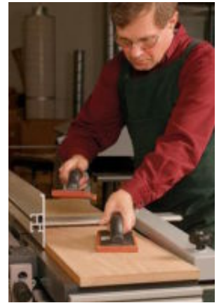
Crossing the bridge. The Hammer and the Rojek have a T-shaped guard. It takes a little practice to learn to maneuver over the guard when jointing.
