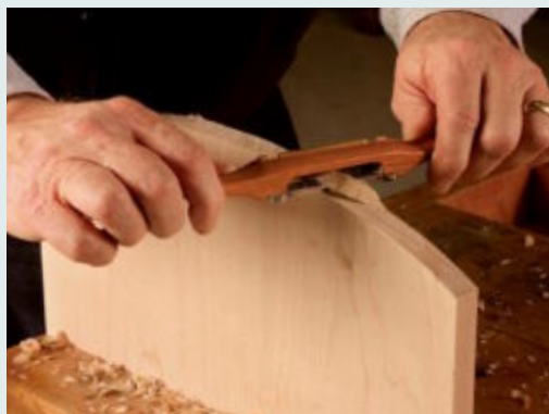
Easy sailing on end grain. The Woodjoy low-angle shave leaves a smooth surface in its wake.
