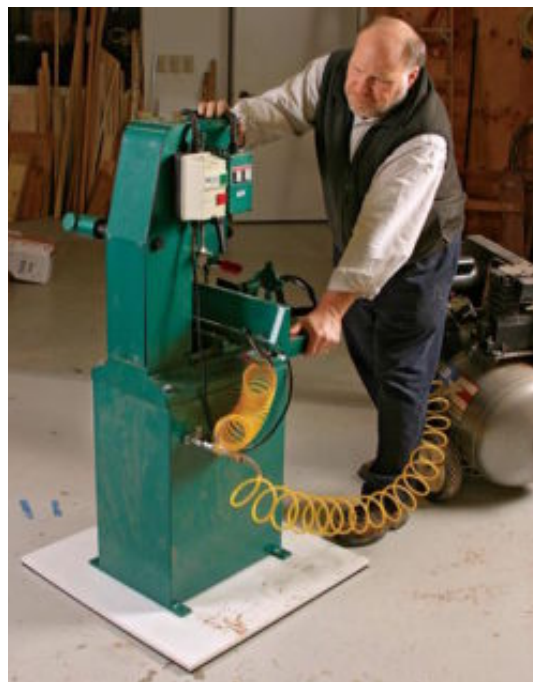
Clear for takeoff. Quick-connect fittings connect the pad to the compressor. Place the machine on the pad and fire up the compressor. In seconds, the machine levitates on a cushion of air.
