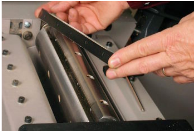
Pretty quick change. Double-edged cartridge knife inserts are easy to change and reset without having to make lots of tiny adjustments.
