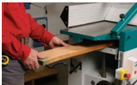
Hangover. The Rojek's jointer table limits your access and view when planing.
