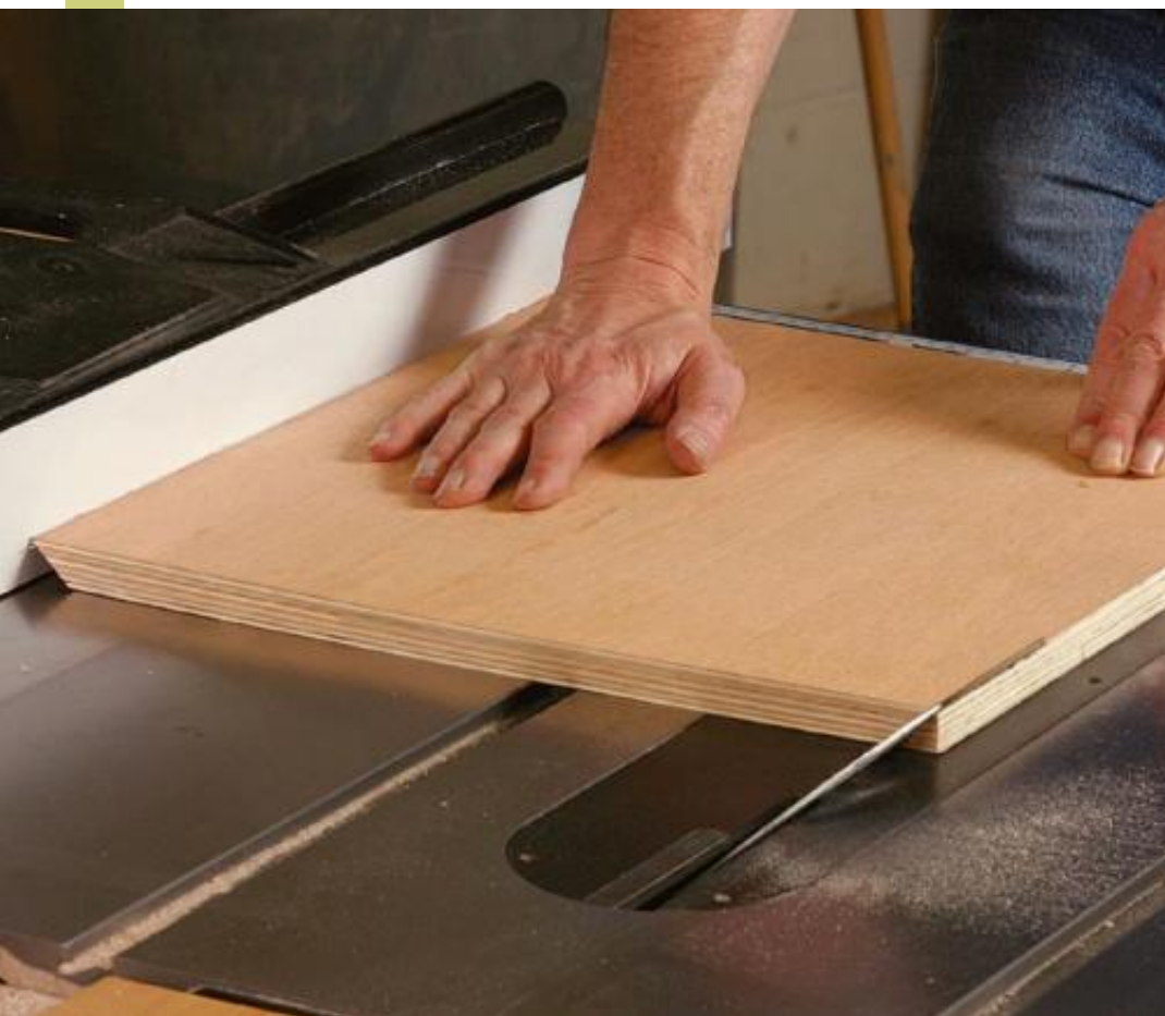
Simple on a left-tilt saw. Here, the thin point of the first miter runs against the rip fence.
