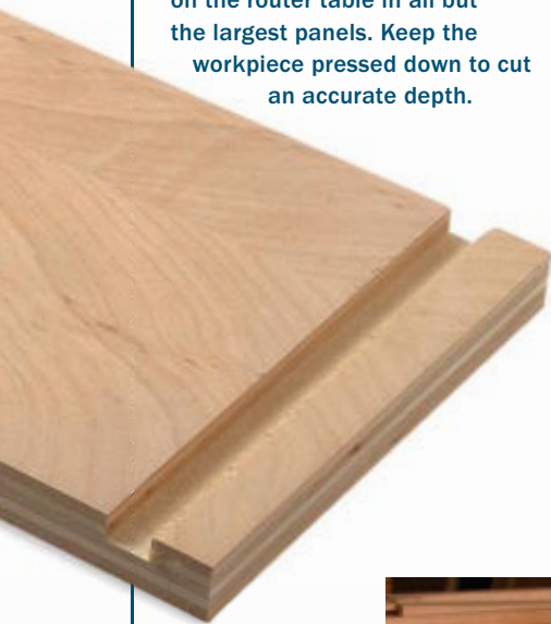
Router fence keeps dado cuts straight. For dadoes that are near the edge of a workpiece, use the fence to guide a clean and straight cut.
