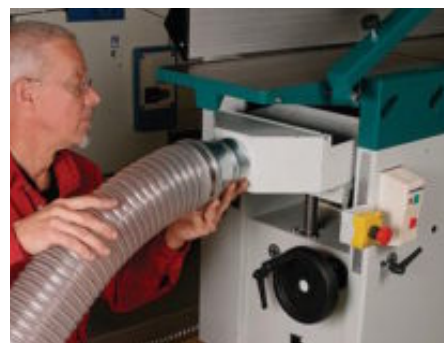
Dust collection one. For jointing, the dust hood fits underneath the cutterhead and is clamped in place by the planer table.
