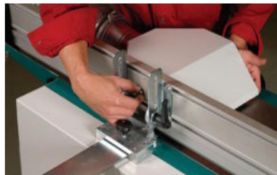
Hangover. The Rojek's jointer table limits your access and view when planing.
