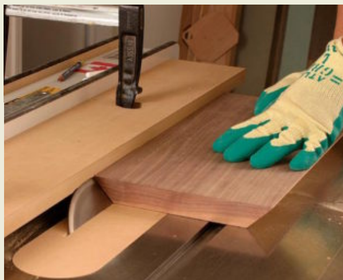
Using a right-tilt saw. When cutting the miter on the second side, to prevent the thin point of the first miter from burrowing under the rip fence, attach a sacrificial fence and cut the miter as shown. Hyatt uses a rubberized glove for better control.
