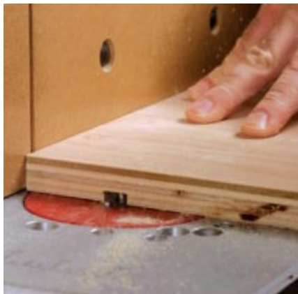
Router fence keeps dado cuts straight. For dadoes that are near the edge of a workpiece, use the fence to guide a clean and straight cut.
