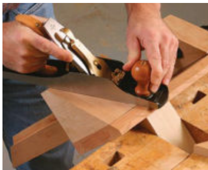
Master the miter. Use the shoot to true up parts for miter joints. The base prevents tearout on the outside edges.
