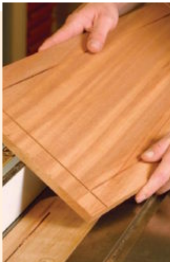
Begin at the shoulder. Make a \frac{3}{16} -in.-deep cut on all four sides using the tablesaw.
