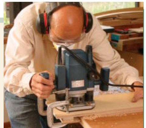
Flush-cut edge-banding. This jig allows you to cleanly cut solid-wood edge-banding flush with a plywood panel.
