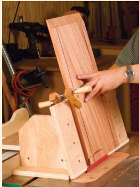
Begin at the shoulder. Make a \frac{3}{16} -in.-deep cut on all four sides using the tablesaw.
