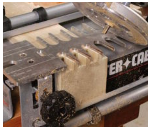
Finished pins. The straight bit supplied with the jig cuts the pins. Here, too, scrap backs up the cut to prevent tearout.
