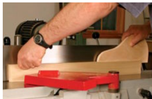
Use a pair of push blocks for face-jointing. It's best to have a non-skid block at the board's leading edge and a cleated block at the rear.
