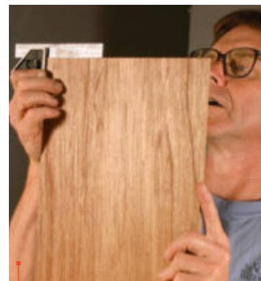
3 Check the cut with a square. Any gaps will help you determine the direction and amount of adjustment the fence requires.
