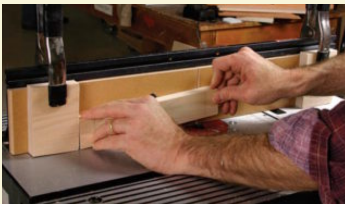
Start and stop. A pair of blocks clamped to a router-table fence makes it possible to begin and end a stopped groove. The blocks help steady the work as you lower and then raise it.
