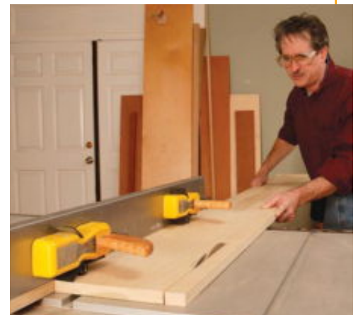
Grip-Tite magnetic hold-downs stick to a steel auxiliary fence.
