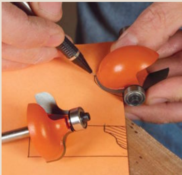
Make templates. Trace the profile of each router bit on thin cardboard to create templates for the molding.
