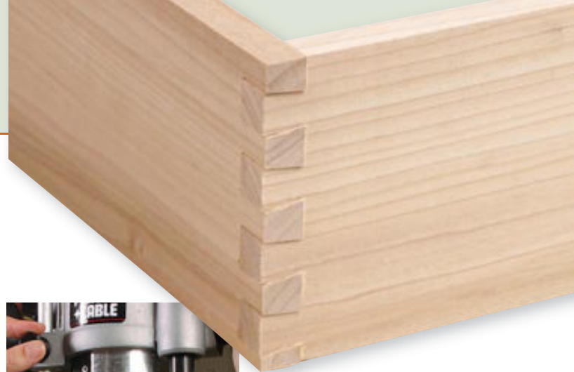
The wood guides the depth. The workpiece thickness determines bit depth. Set the bit a hair past the edge of the board, leaving the pins slightly proud. They can be trimmed flush later.
