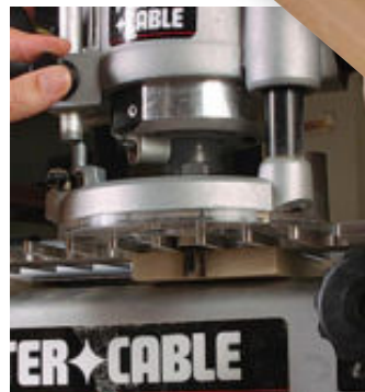
The wood guides the depth. The workpiece thickness determines bit depth. Set the bit a hair past the edge of the board, leaving the pins slightly proud. They can be trimmed flush later.
