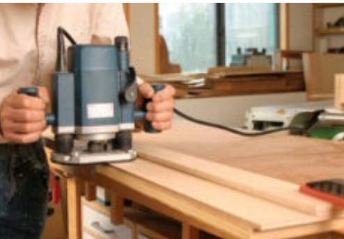
Straighten edges. Rough-cut the panel, then clean up the cut with this straight-edge jig.
