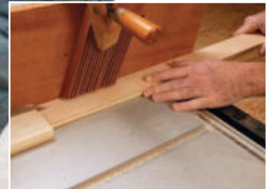
Sacrificial push stick works with hold-downs in place.
