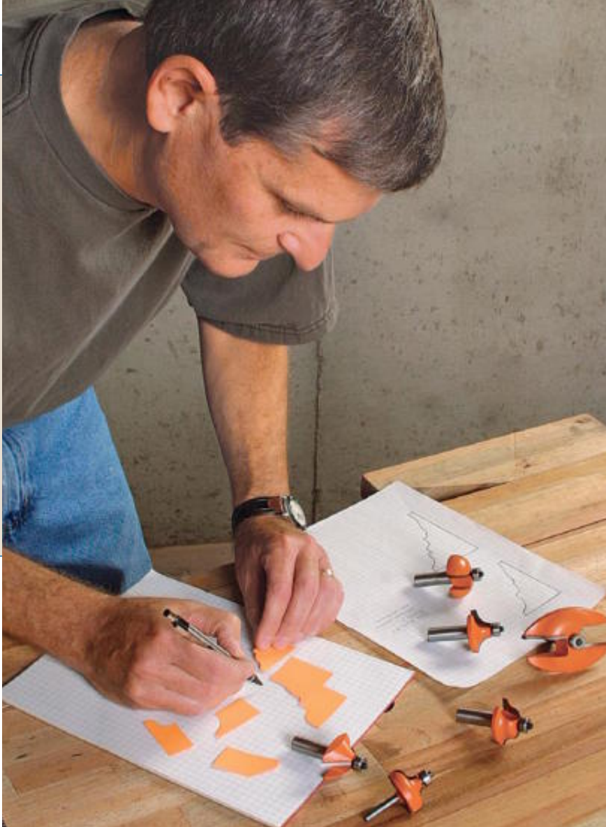
Make templates. Trace the profile of each router bit on thin cardboard to create templates for the molding.
