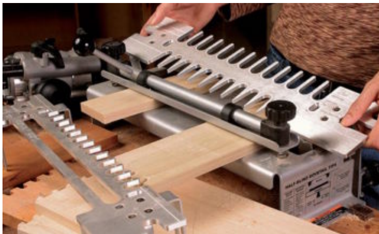
Through-dovetail template. Through-dovetails require a double-sided template and two router bits. The straight fingers guide the router to cut tails; the tapered fingers guide the cut for pins.
