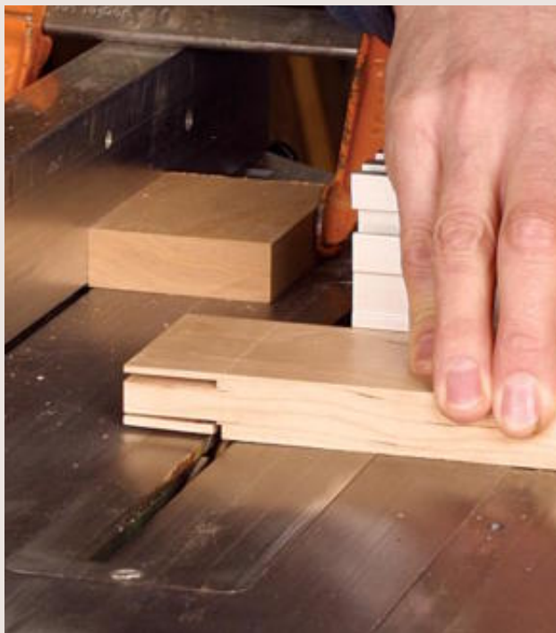
Use the miter gauge and a stop block. For consistent tenon shoulders, clamp the stop block to the rip fence and make the shoulder cuts using a miter gauge.
