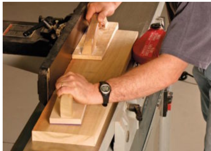
Use a pair of push blocks for face-jointing. It's best to have a non-skid block at the board's leading edge and a cleated block at the rear.
