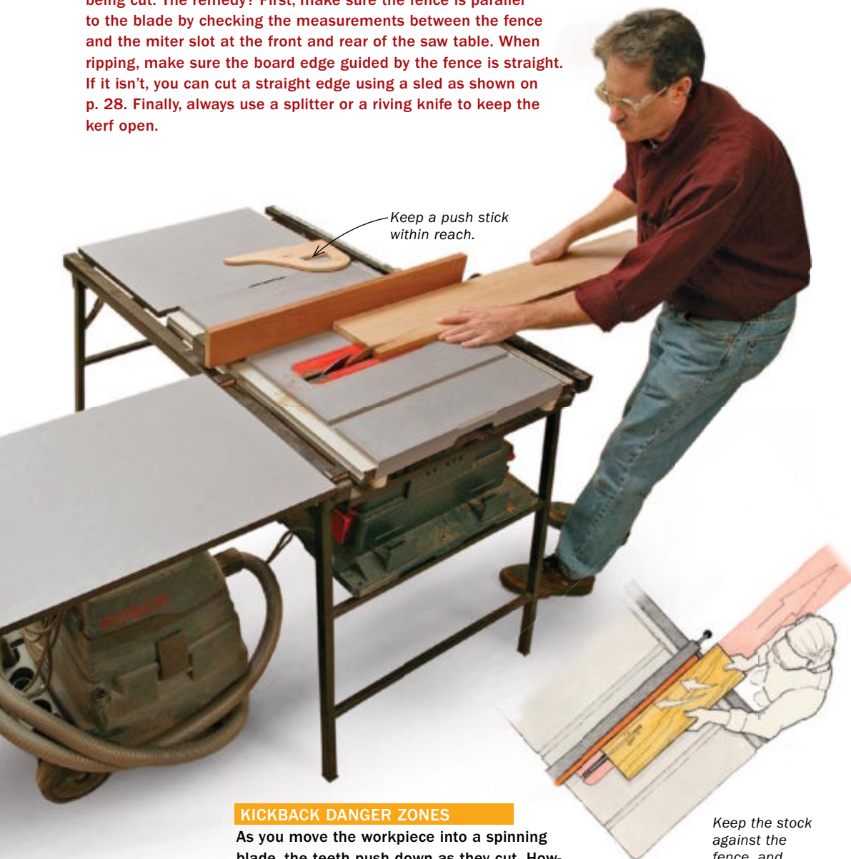
Keep the fence parallel to the blade.
