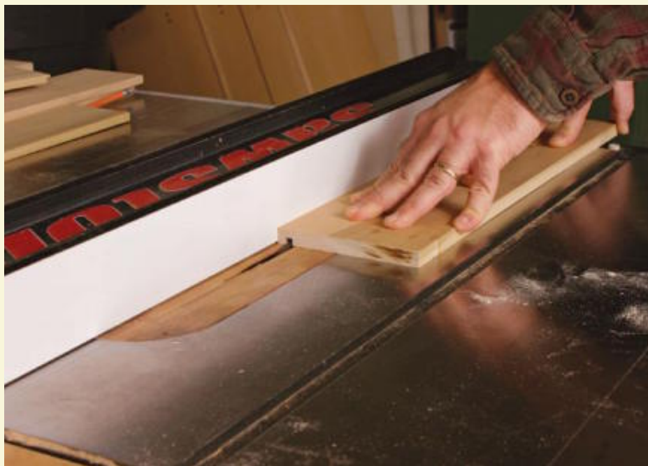
Steady pressure. When cutting grooves or rabbets, press down on the workpiece to ensure that the cut has a uniform depth. Keep hands away from the blade's exit point.
