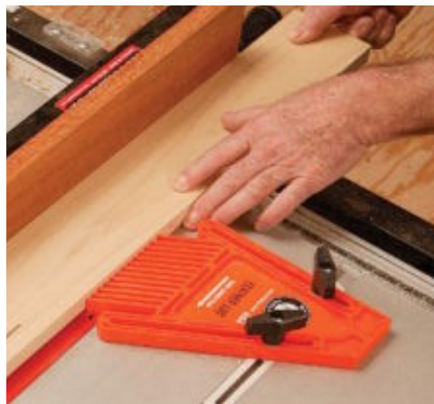
Bench Dog featherboards ride in the miter-gauge slot.
