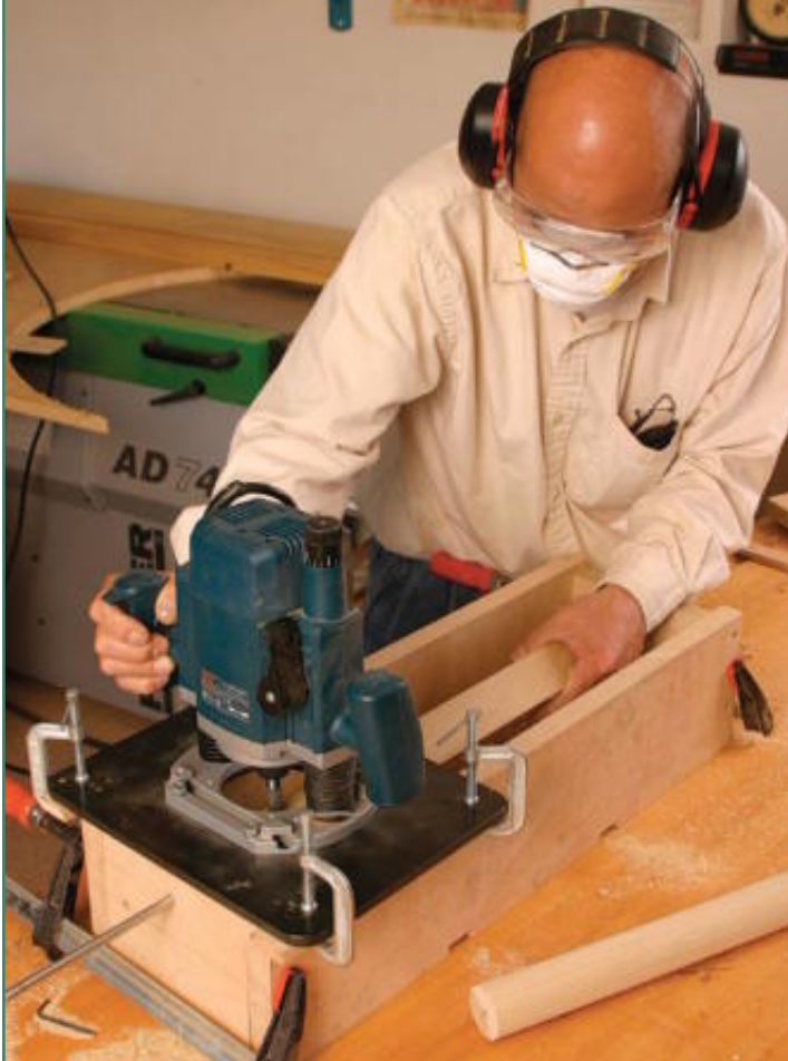
Router-cut turnings. By guiding the router back and forth while turning the workpiece, a square blank gradually becomes a cylinder.
