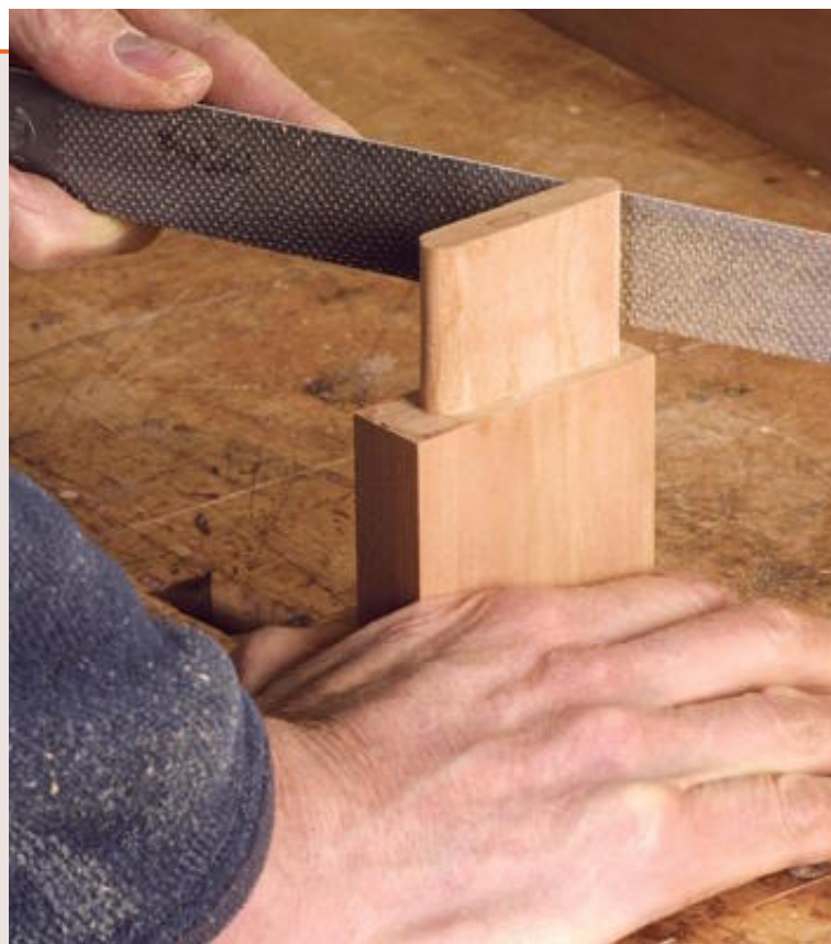
Finish the tenon by hand. Use a rasp to round over the edges of the tenon to match the mortise, then chamfer the end to minimize glue squeeze-out.
