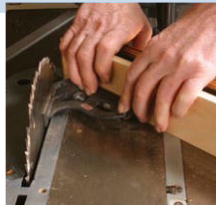
Putting the miter in miter gauge. Use just the head of the combination square to set a miter gauge for an accurate 45° cut.
