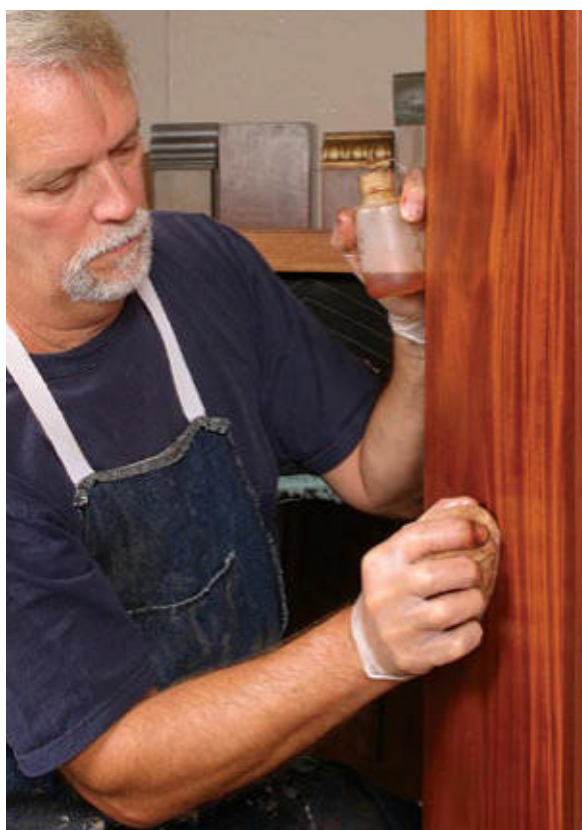
Seal the wood. Go over the surface a couple of times with a pad to apply a thin coat of shellac. Keep the pressure light to avoid filling the pores. It is easier to get into corners, carvings, and moldings by applying the shellac with an artist's brush (above).
