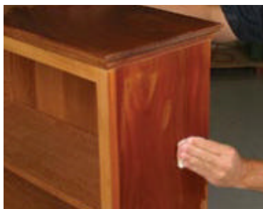
Reading the wood. To get an idea of what the wood will look like under a clear finish, wet the surface with denatured alcohol.
