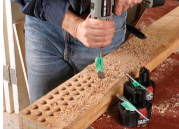
Brutal test. To test the rebuilt batteries, we used a spade bit to drill 1\frac{1}{4} -in.-deep holes into white oak.
