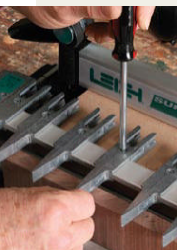
Adjustable tails and pins. Sliding fingers allow users to create any dovetail spacing. A square-drive screwdriver (supplied) secures them.
