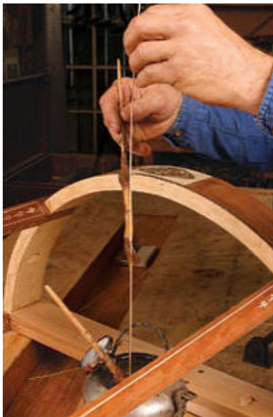
Apply hot glue and press it in place. Be sure the inlay is sized correctly, and then brush glue onto it.
