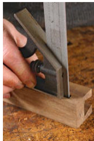
Check mortises and tenons. Adjust the ruler to the desired depth and set it into the mortise (left); if the head doesn't touch the surface, the mortise is too shallow. A square can also help check whether tenon cheeks are parallel to the face of the workpiece (right).
