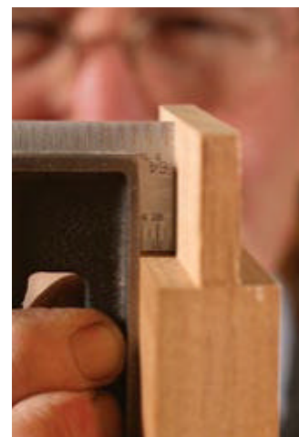
Check mortises and tenons. Adjust the ruler to the desired depth and set it into the mortise (left); if the head doesn't touch the surface, the mortise is too shallow. A square can also help check whether tenon cheeks are parallel to the face of the workpiece (right).
