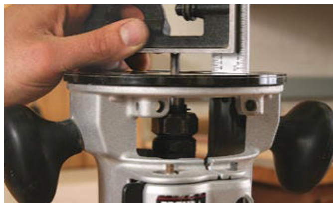
An adjustable height gauge. Set the head at the desired measurement. Hold the end of the ruler flat against the router's base and raise the bit until it touches the head without lifting the ruler.
