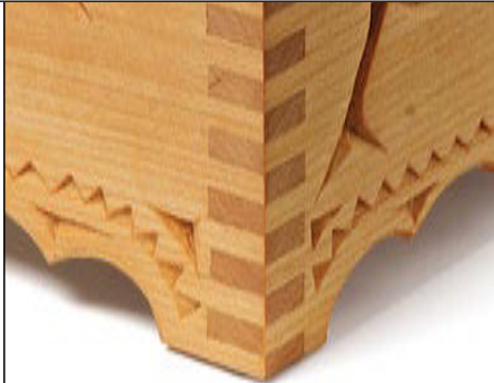
Cutaway sides. By cutting away the bottom edge of the sides, the box effectively ends up with four feet.
