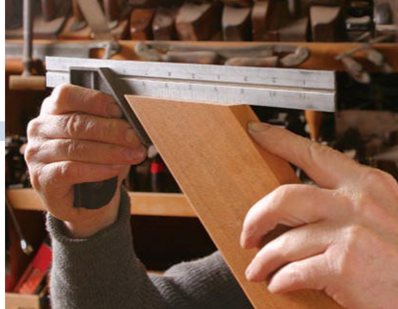
Checking for square and the trueness of a miter. First, set the head of the square against the reference surface, then lower it until the ruler touches the highest point (left). Face a light source and look for a gap under the ruler.
