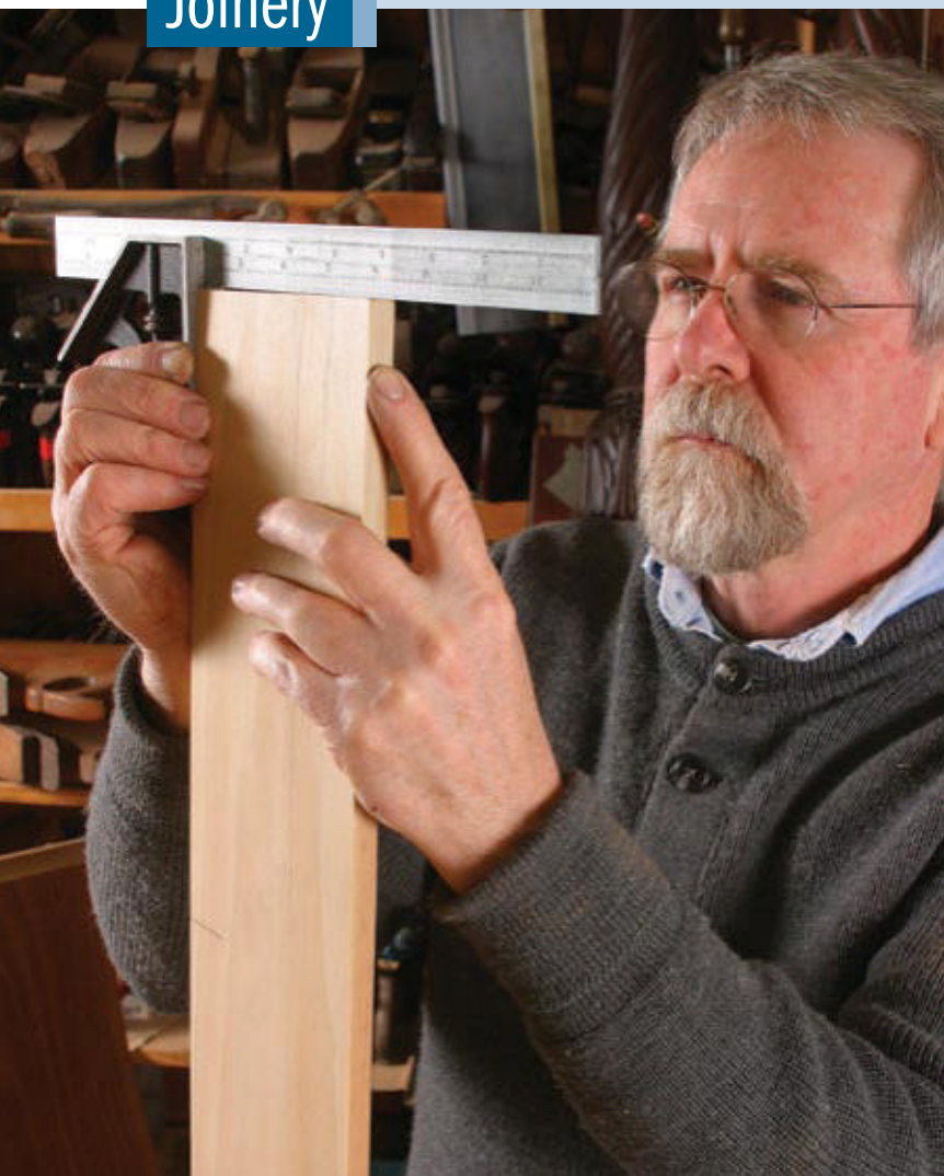
Checking for square and the trueness of a miter. First, set the head of the square against the reference surface, then lower it until the ruler touches the highest point (left). Face a light source and look for a gap under the ruler.
