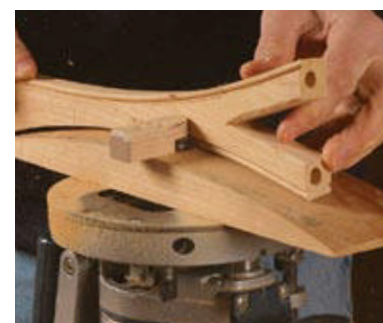
Beaded by router. Simple jigs attached to a router base allow you to bead the Xs quickly and cleanly.
