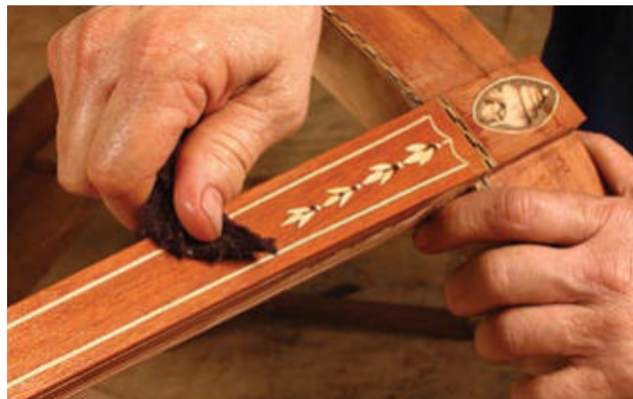
Easy cleanup. After a few minutes, dampen a scrubbing pad with warm water and remove the excess glue.
