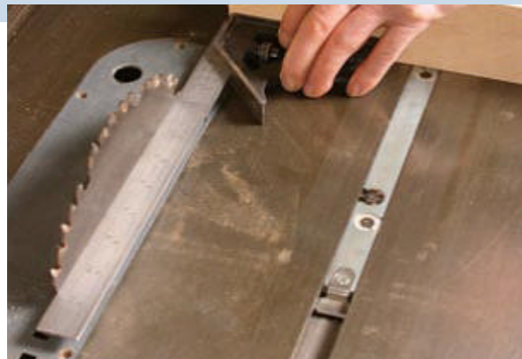
Setting up for square crosscuts. Hold the combination square with its head against the miter gauge. Adjust the gauge until the square's ruler rests flush against the side of the sawblade. This ensures a 90° crosscut.
