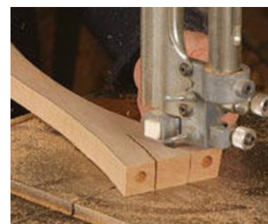
Curve the slats. Cut the curved side profile of the slats on the bandsaw (left). Then bandsaw the X design on each of the slats (above).
