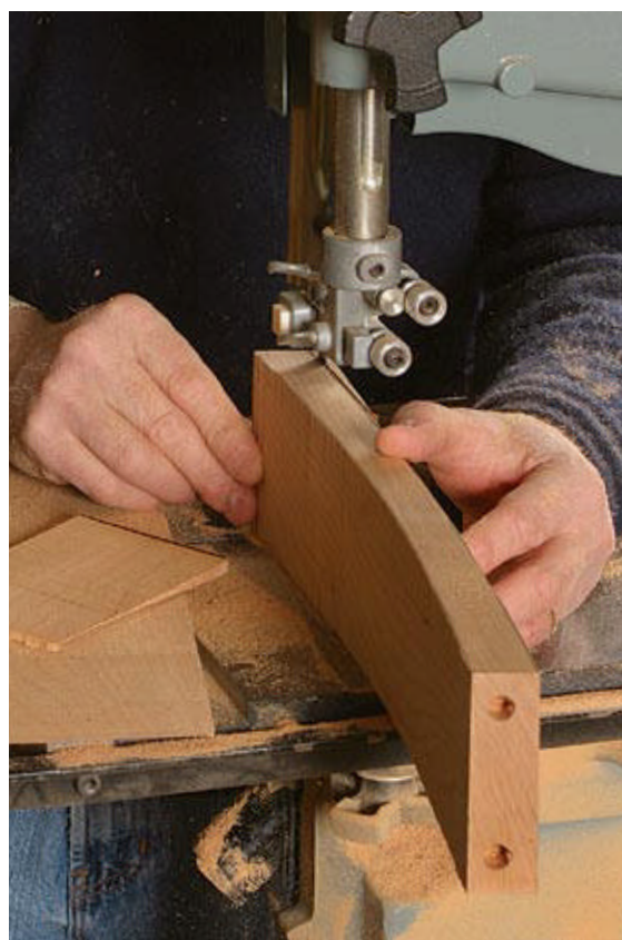
Curve the slats. Cut the curved side profile of the slats on the bandsaw (left). Then bandsaw the X design on each of the slats (above).
