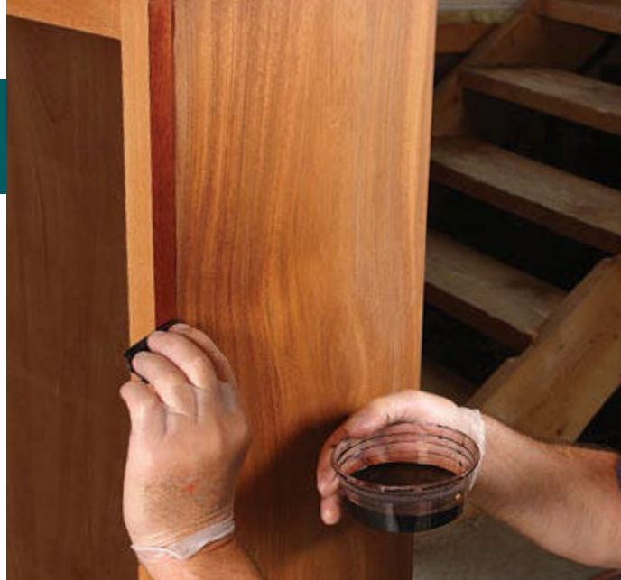
Harmonize the color. To merge the pale face frame with the rest of the piece, Gedrys applies a water-based dye using a folded paper towel. Look ahead of your hand to get a nice, straight line.
