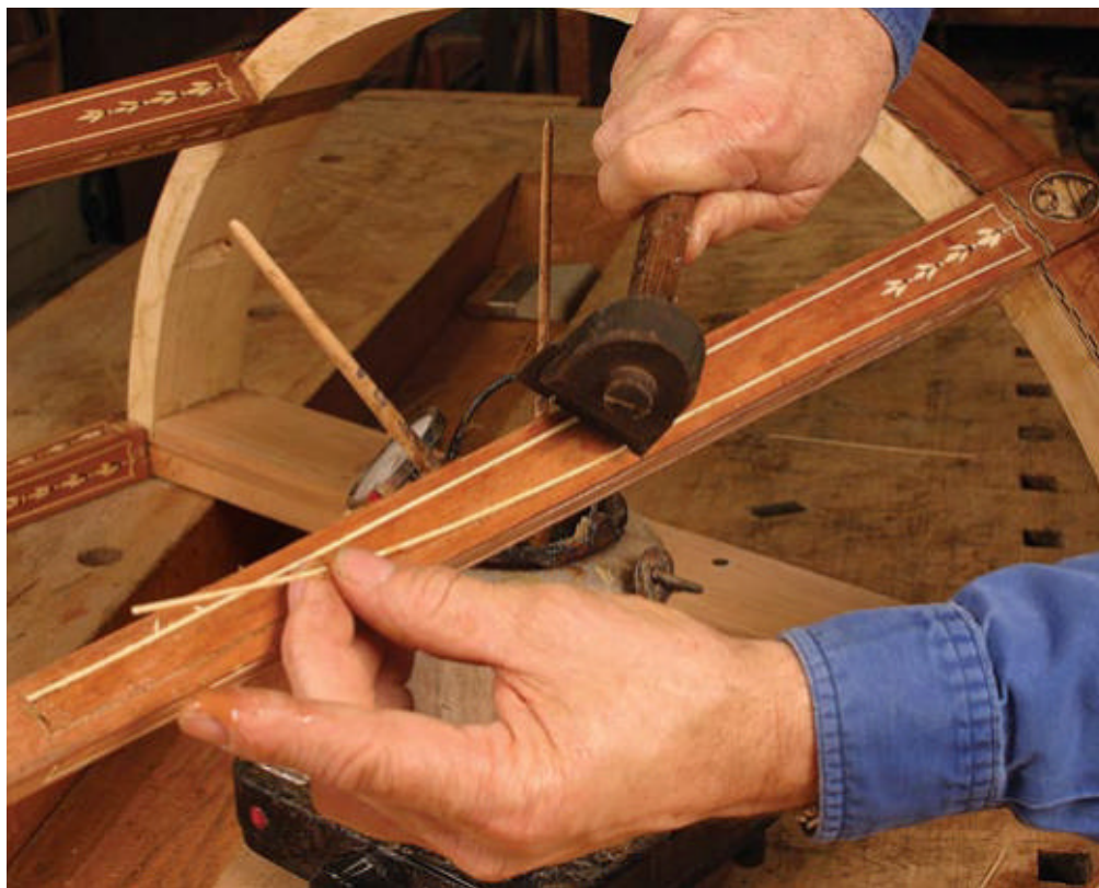
Press it in place. Edwards uses a veneer hammer to push stringing evenly into its groove.
