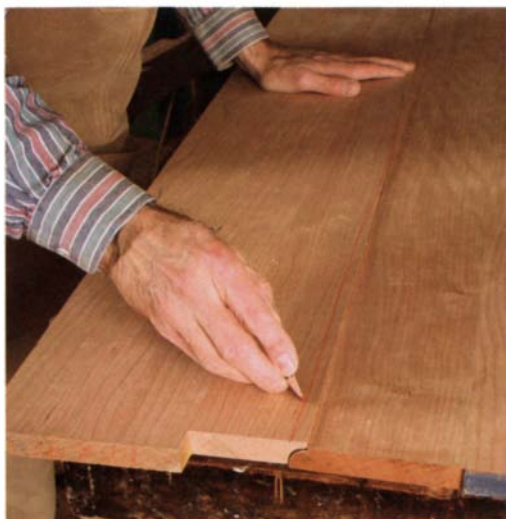
Mark the contact spots. Set the leaf in place, and mark spots where the joint makes contact.
