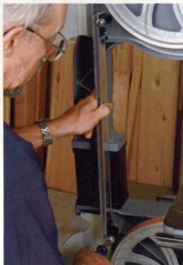
Attach the replacement blade guards and the guidepost. The riser-block kit includes longer blade guards for both the back and front of the saw, and a longer guidepost.
