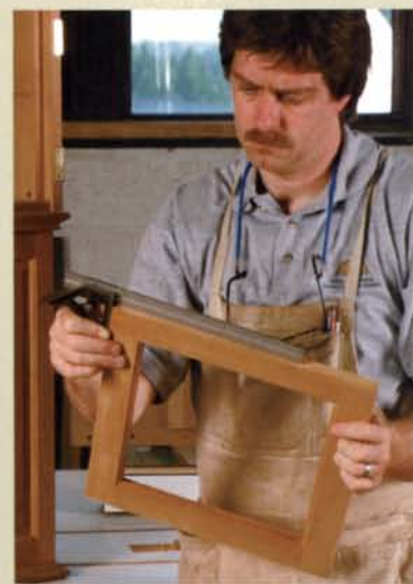
Checking a frame for square
