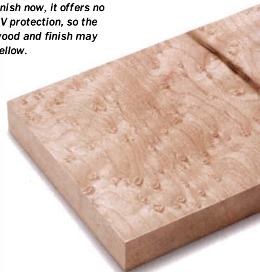
Clear finish with no yellowing. A water-based acrylic is easy to apply and remains clear over time, but it brings little depth to the grain.
