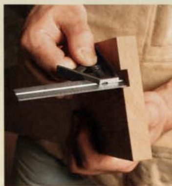
Checking the depth of a groove
