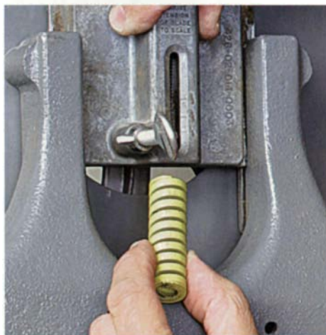
Replace a worn-out spring. If your cut wanders, chances are that the spring is not providing enough tension to the blade.
