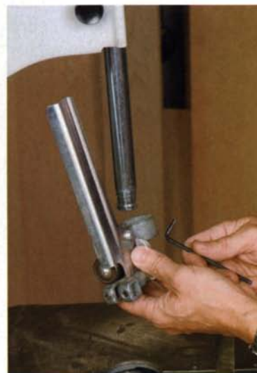
Attach the replacement blade guards and the guidepost. The riser-block kit includes longer blade guards for both the back and front of the saw, and a longer guidepost.
