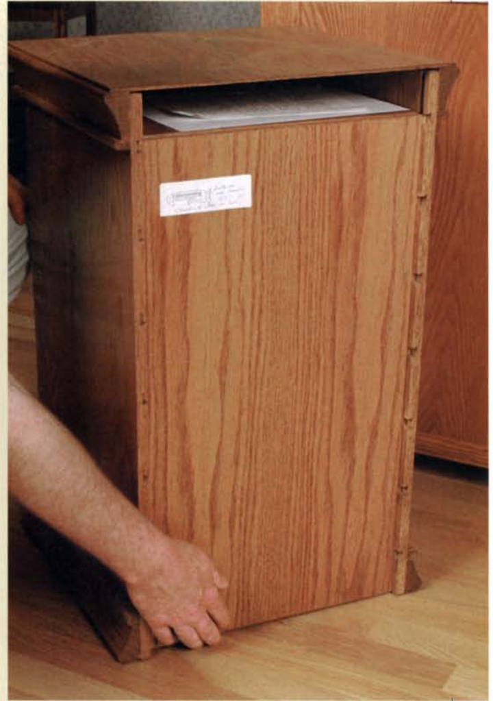
A hidden catch. The rear of the spice cabinet has a bar on which the back panel rests. When pushed, the back panel slides down to reveal a compartment that's hidden behind the cornice molding.
