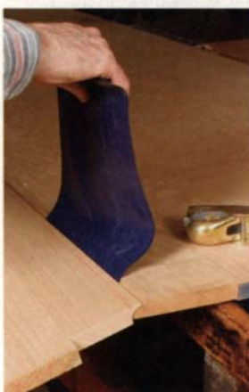
Carbon paper still has a use. Becksvoort holds carbon paper between the joint as he opens and closes the leaf. Black marks are left where the joint is too tight. Those spots are trimmed with sandpaper or a block plane.
