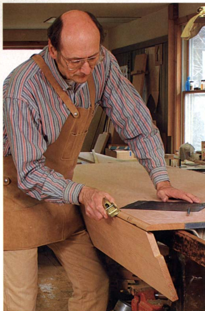
Carbon paper still has a use. Becksvoort holds carbon paper between the joint as he opens and closes the leaf. Black marks are left where the joint is too tight. Those spots are trimmed with sandpaper or a block plane.
