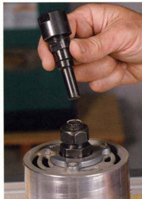
Collet stretcher. The router-collet extension from MLCS adds about 2\frac{1}{4} in. to the length of a router collet, a handy feature in the router table for above-the-table bit changes.
