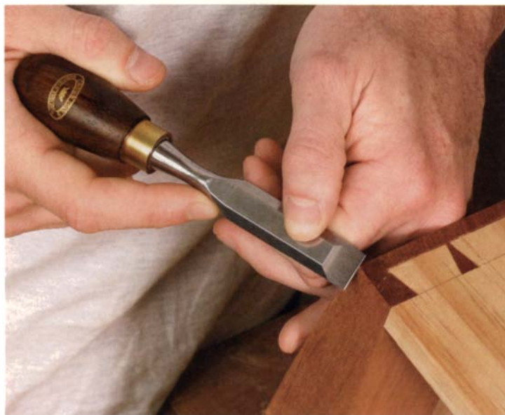
Compact chisels add control. With short blades and small handles, butt chisels are perfect for working in close quarters.
