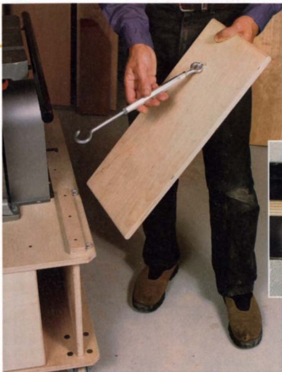
Supports assemble in seconds. Mounting the infeed and outfeed supports is simple. One end butts against a stop, and the other hooks to the underside of the saw table.
