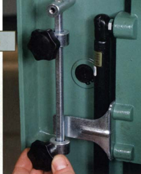
Stop systems set the depth of cut simply by stopping the travel of the mortise head. The Bridgewood, Geetech, Grizzly, Woodtek and Powermatic use a sliding stop that's secured with a lock knob (left). The General incorporates a threaded rod with lock collars (right).
