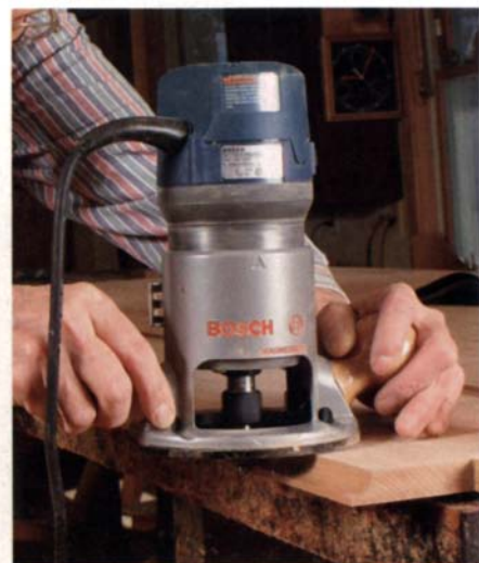
Trim the leaf, not the tabletop. A few passes with a handplane helps achieve an even reveal. Once the joint closes up, rerout the profile on the leaf and try another test fit.
