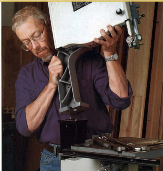
The riser block mounts between the upper and lower frames of the saw. Two pins help position the block on the frame. All three parts are held together with a heavy-duty bolt, washer and nut.
