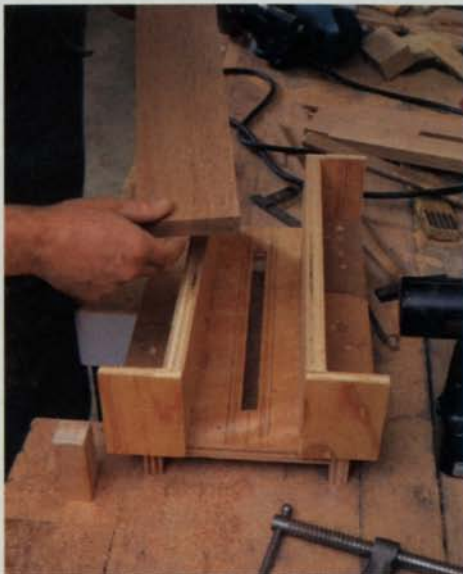
1. Movable base supports make adjustments easy. Built for mortising a set of doors, this jig can be adjusted to cut mortises in stock of different widths.
