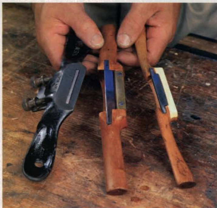
Preventing wear—Spokeshaves used to wear quickly in front of the blade. To prevent this, manufacturers turned to wooden wear plates, usually boxwood. Brass wear plates were an improvement, and metal spokeshaves eliminated the problem.
