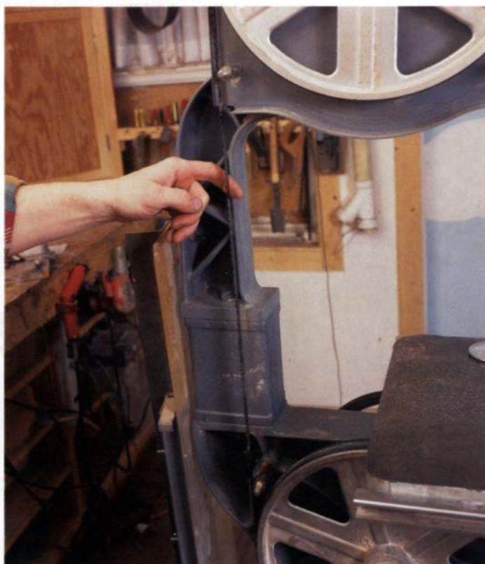
Pluck the blade to check the tension. Listen for a clear note, roughly an E on a bass guitar. The author replaces the blade guard after tensioning the blade.
