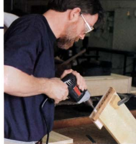
Doweling jig —Holes bored in a hardwood scrap guide the bit as the author drills out a case side for glue dowels.
