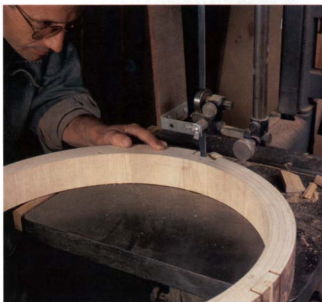
Forming the leg sockets —The author starts on a tablesaw, using a miter-gauge jig to cut the ends of a half-lap joint for each leg (above). A bandsaw removes the rest of the waste (right).
