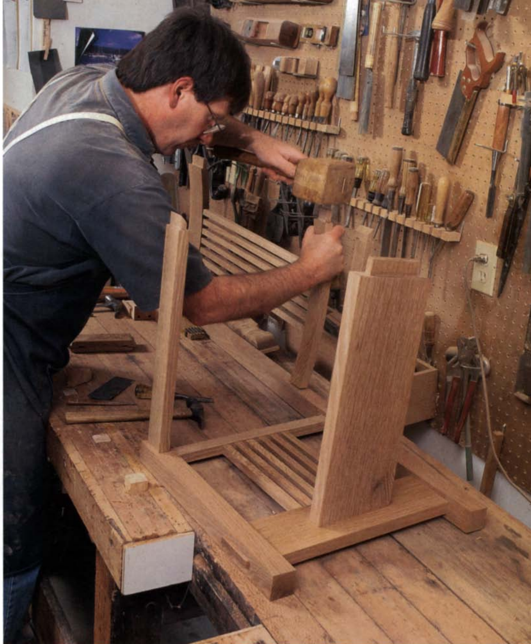
Dry-assemble all the pieces. This dress rehearsal for the final assembly helps the author avoid the costly mistake of glued joints that don't fit.
