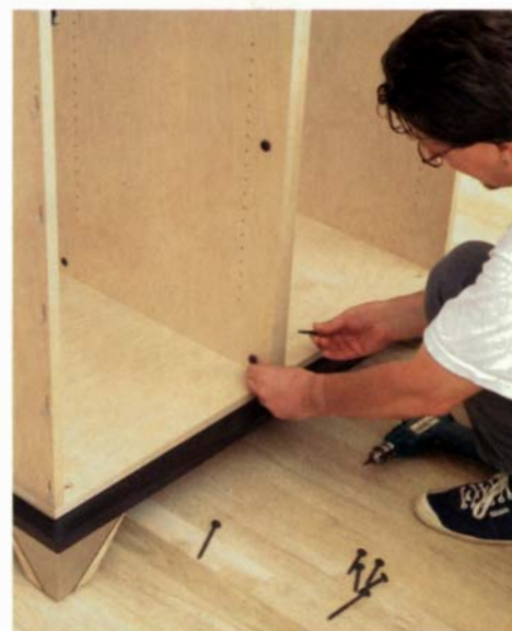
Hex-drive connector bolts and threaded sleeves—This hardware is ideal for linking adjoining carcasses.
