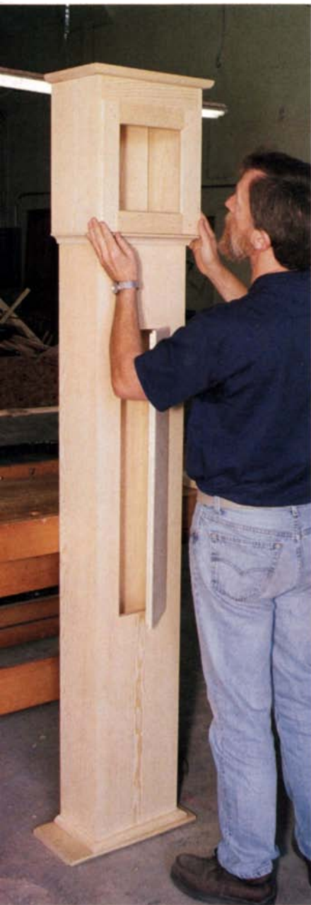
Slide-on bonnet —The bonnet for this Shaker tall clock rests on transitional molding at the top of the case. It slides on and off to provide access to the clock's movement.
