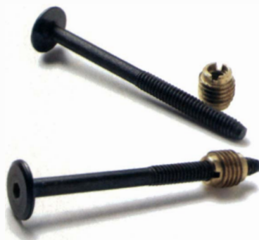
Hex-drive connector bolts and threaded inserts fasten cabinet parts together where connector heads can be exposed. The connector at right secures a cabinet carcass to its base.
