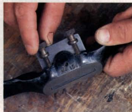
Knurled nuts allow precise adjustment. Because there are two posts, the blade can be skewed so that one side takes a fine cut and the other a heavy cut.
