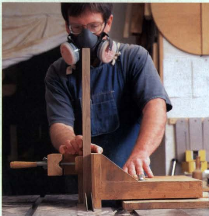
Double-blade tenoning on the tablesaw —With a custom-made jig, the author cut angled tenons for the side stretchers and side seat rails. Sawblades were set at a 4^\circ pitch to the surface of the saw table and separated by a \frac{1}{2} -in. spacer.
