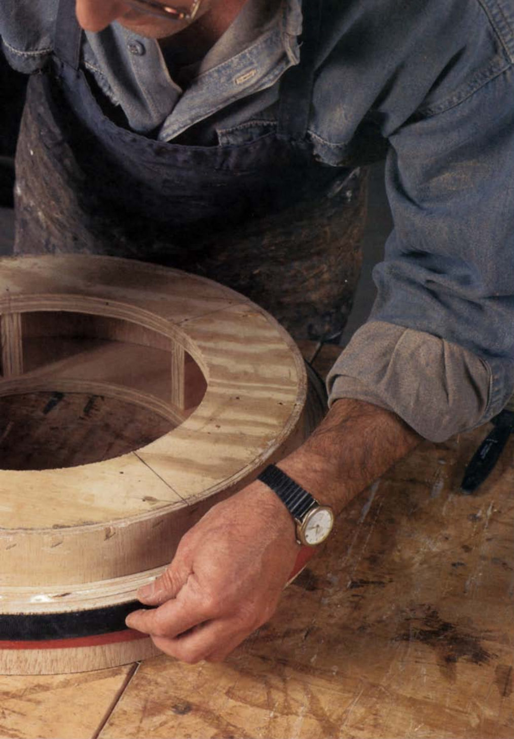
Bendable plywood —The author uses Wiggle Wood to make circular table aprons. The wood comes in 4x8 sheets, either \frac{1}{4} in. or \frac{3}{8} in. thick.
