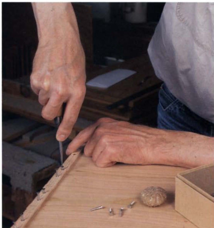
Countersink holes, and then screw the keys down. A little beeswax applied to the screw threads will make the job easier and reduce the chance of a screw breaking.
