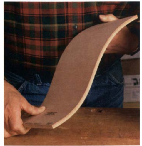
Bendable plywood —The author uses Wiggle Wood to make circular table aprons. The wood comes in 4x8 sheets, either \frac{1}{4} in. or \frac{3}{8} in. thick.
