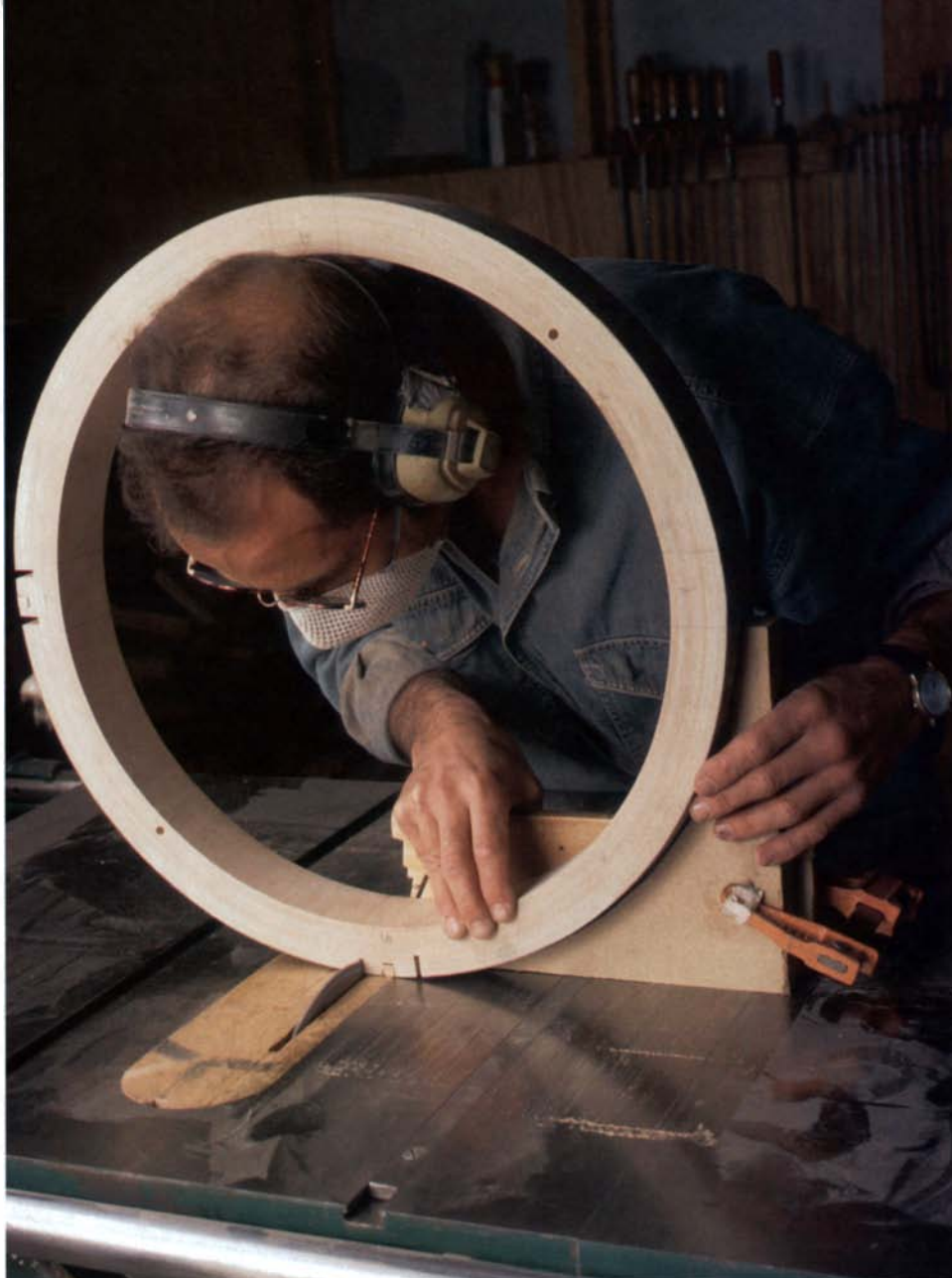
Forming the leg sockets —The author starts on a tablesaw, using a miter-gauge jig to cut the ends of a half-lap joint for each leg (above). A bandsaw removes the rest of the waste (right).
