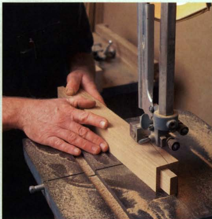
Cutting the curved back slats —Convex and concave cuts from 8/4 lumber yielded \frac{7}{8} -in.-thick slats, after the surfaces were scraped clean. These slats are the only curved pieces of the chair.
