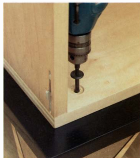
Hex-drive connector bolts and threaded inserts fasten cabinet parts together where connector heads can be exposed. The connector at right secures a cabinet carcass to its base.
