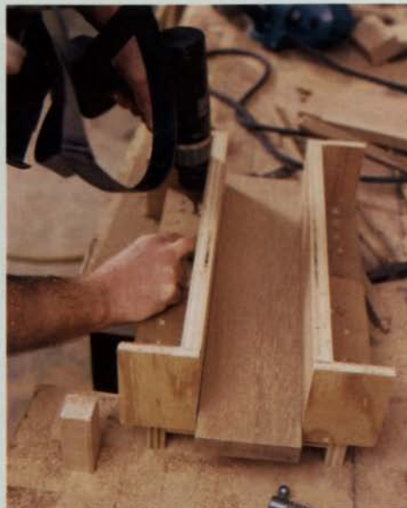
2. Use chair part to set jig. After securing one base piece, the author snugs the other one against a side stretcher and screws it in place.
