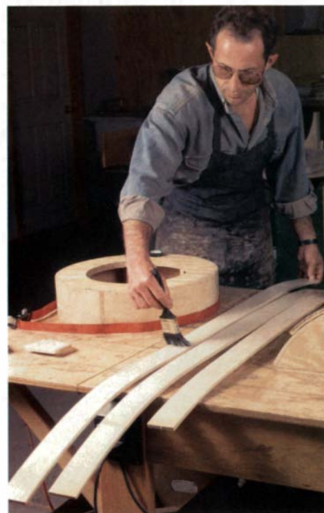
Three layers of plywood are painted with thinned glue and then wrapped and clamped on the form at left.
