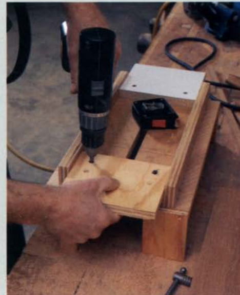
3. Stop blocks for the router determine the length of the mortise cuts and keep them all consistent. Pencil lines help to align the stock.
