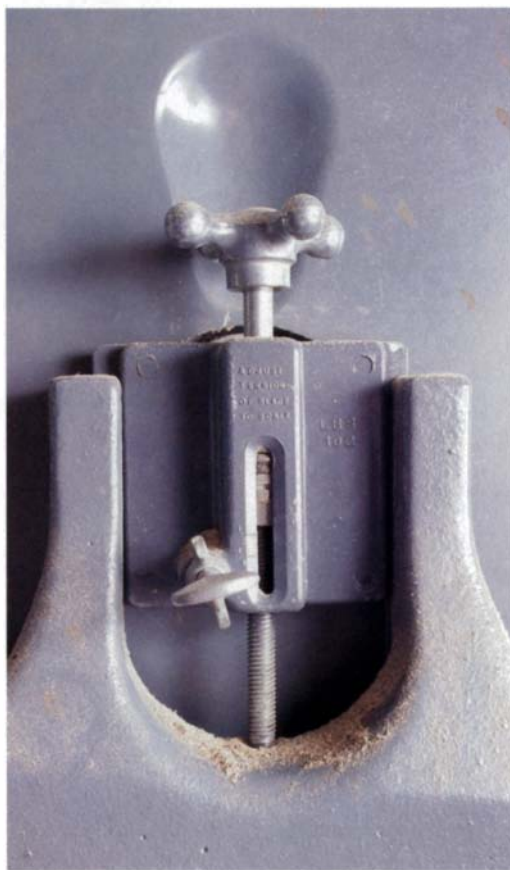
Blade-tension scales aren't exact. The author tensions the blade by ear, not by the calibrations on the saw.
