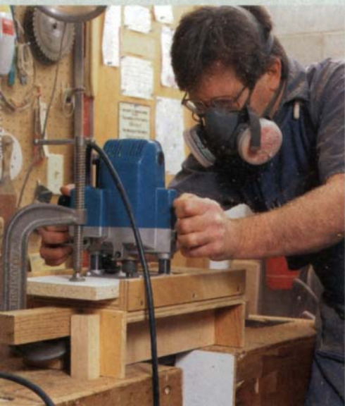
4. The depth of the mortise is controlled by the plunge mechanism on the router. The author secures stock to the jig with C-clamps.
