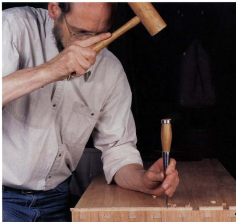
Chop out the waste. The author uses a mallet and a sharp chisel to remove waste between keys. Any chisel marks between keys will be hidden by the molding.
