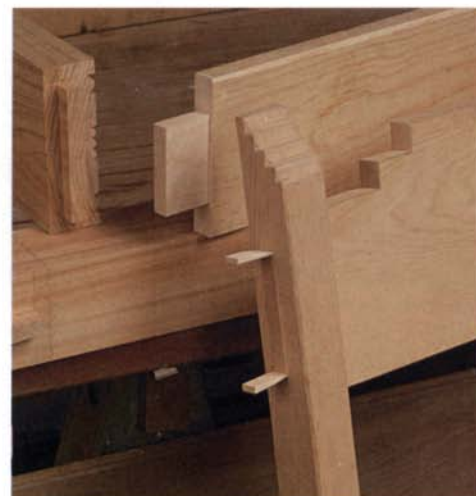
Wedged through-tenons are popular. Unlike common through-tenons that have wedges near the middle, end-wedged tenons are typical of New Mexican furniture.
