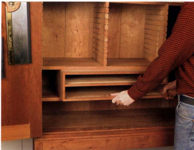
Oversized storage holds big items — This two-drawer box slides into place between the shelves to hold long items that don't fit in the smaller drawers.
