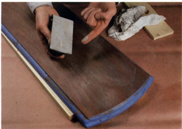
Sand down to the wood (or sealer) once the filler is dry. Minick uses 120- and then 220-grit paper to produce the fine powder shown. If the paper starts to gum up, it means the filler is not quite dry.
