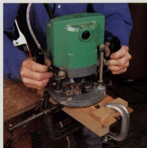
Quick and simple mortising jig, p. 82
