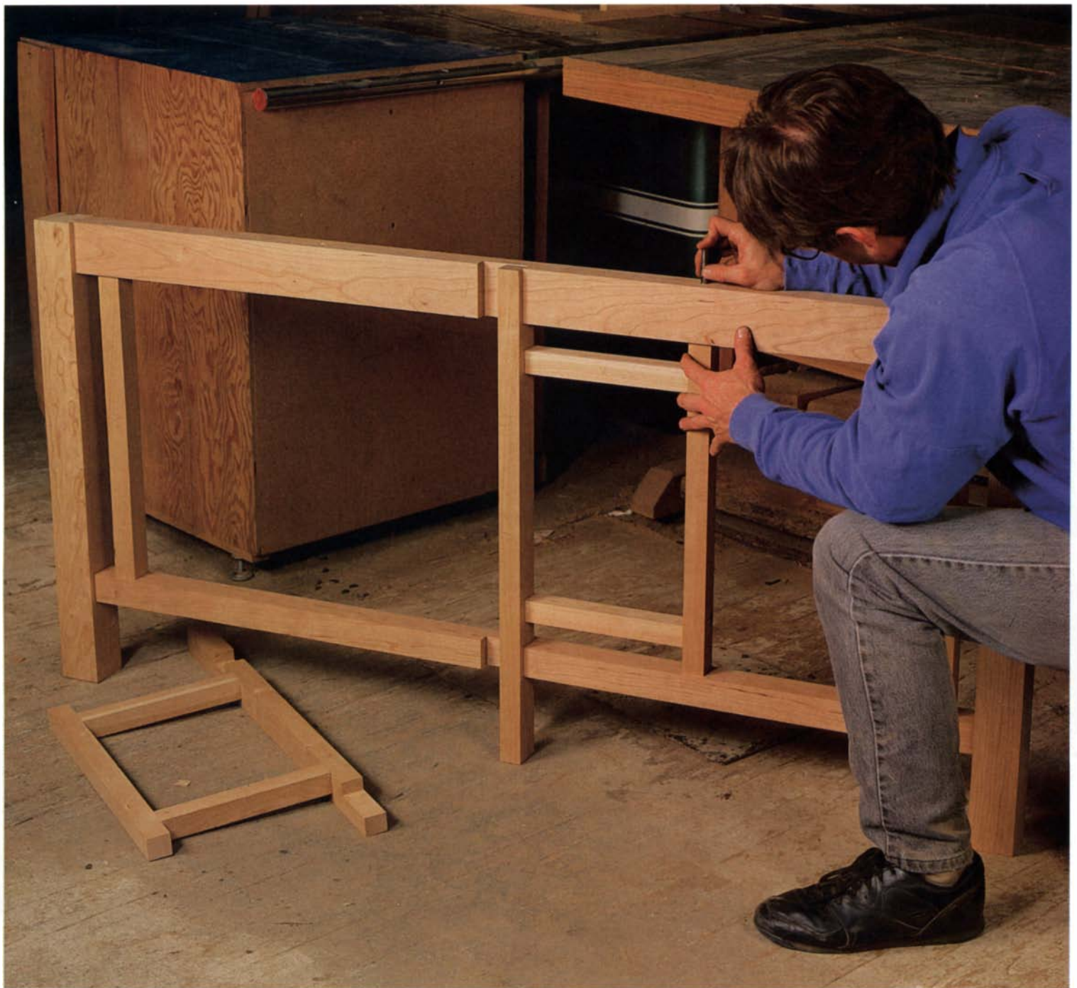
Drill bit marks pivot point. After trimming pivot posts to size and checking the fit of the gates, the author marks where he'll drill for the bushing and hinge pin. He drops a drill bit through the bronze bushing in the rail to make a mark.
