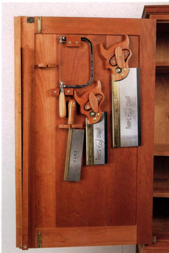
Preventing door sag —Legs screwed to the doors' lock stiles help support the heavy tools hung on the doors and prevent the hinge screws from pulling out.
