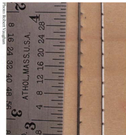
Precision grinding and six reversed teeth prevent tearout. Olson's new PG #459 is a little more delicate than other scrollsaw blades of the same size, but the tearout-free finish it leaves far outweighs its slightly more fragile nature.
