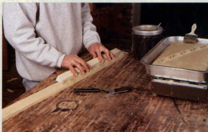
Applying precast moldings is easy, requiring no special equipment and can dramatically transform a case. And the moldings are inexpensive compared to hand-carving the intricate details.
