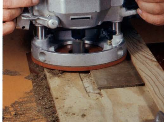
The router jig above is used to trim templates that are the same width as the distance between the router's edge and the cutting edge of the bit.
