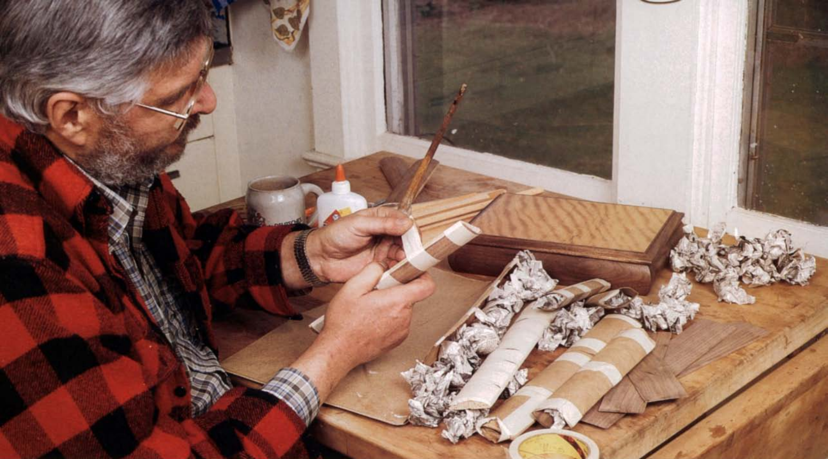
Masking tape is an essential "tool" for building the jewelry box. Above, the author "clamps" the steam-bent veneer to one of the pine box sides. Masking tape was also used to clamp the two pieces of curved molding together to form each side.
