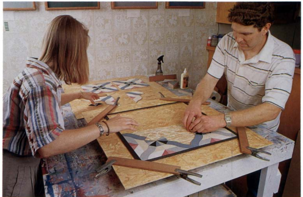
To keep the borders from bowing, they are secured with spring clamps and four, 1/2-in.-thick strips of scrapwood across the corners. The assembly is then covered with Masonite and weighted evenly with 10 lbs. to 15 lbs. per square foot while the glue dries.
