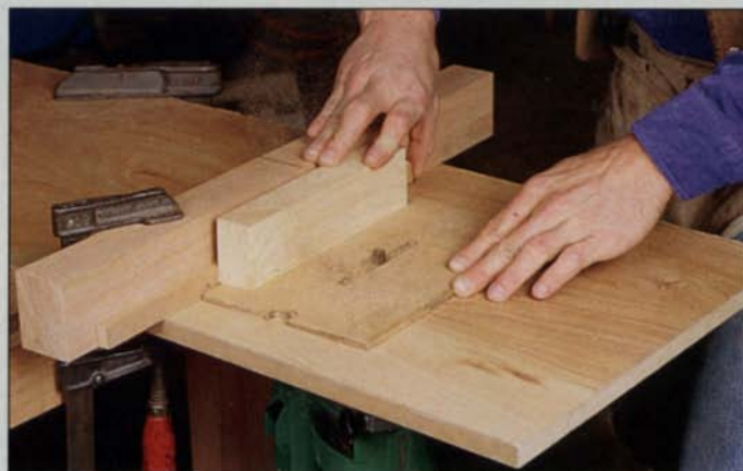
To widen the mortise guide's slot, Rogowski shims between the guide and the router-table fence, moving the guide enough for the spinning bit to cut the inner side of the guide slot.
