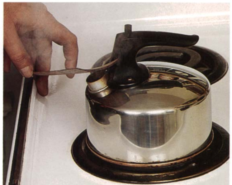
Steaming one side only of shop-cut veneer causes the steamed side to expand, gently curving the veneer along its length. Cummins then slipped the veneer into a paper sleeve to hold the curve.
