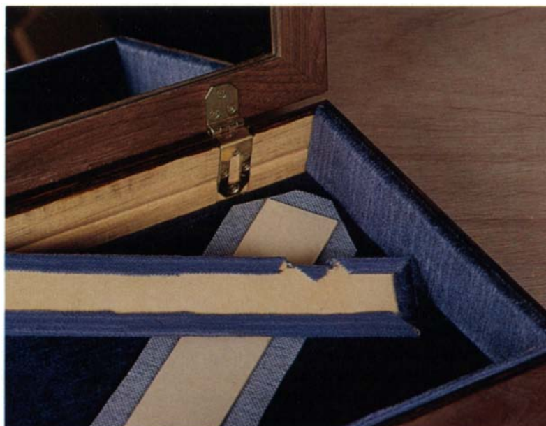
Velvet-covered cardboard strips line the interior of the box and conceal the hinge mortises. The hinges are actually brass hasps from a hardware store. The mortises were made with a series of shallow cuts on the tablesaw before the box was assembled.
