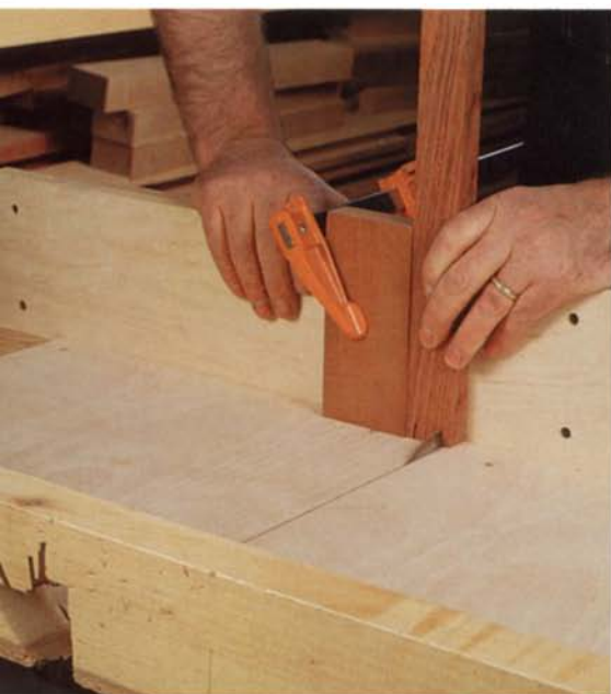
To cut dovetails on the ends of the drawer rails, Moore uses a tablesaw crosscut box and clamps a vertical guide on its fence. Cutting different angles widens the box's kerf, so he renews the box by screwing plywood to the base and fence and cutting a fresh kerf.
