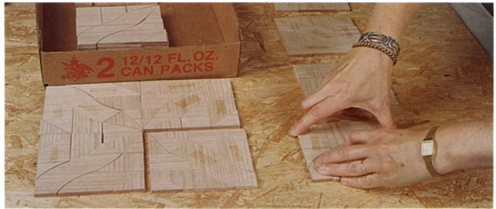
Pieces with different grain directions are interchanged to create texture in the overall quilt. First, the taped blocks are pried apart carefully with a knife. After the tape is removed, individual pieces are laid out into new pattern blocks. Note that all of the pieces of a stack are kept in their original positions in the pattern.
