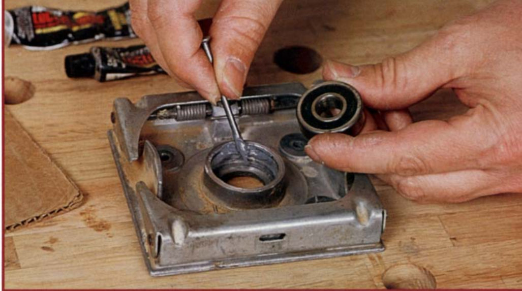
You can build up a worn-out bearing socket, such as the one shown here on the bottom plate of an orbital sander, with fortified epoxy. To do this, give the new bearing a light coat of wax, apply epoxy to the worn socket and set the bearing in place.
