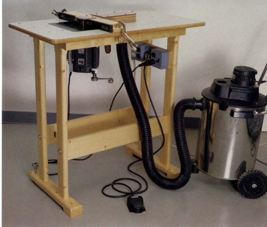
This shop-built router table is sturdy yet lightweight and knocks down for portability. It also has a quick-clamping fence with an adjustable bit opening, a dual-router setup and a built-in dust-collection system.
