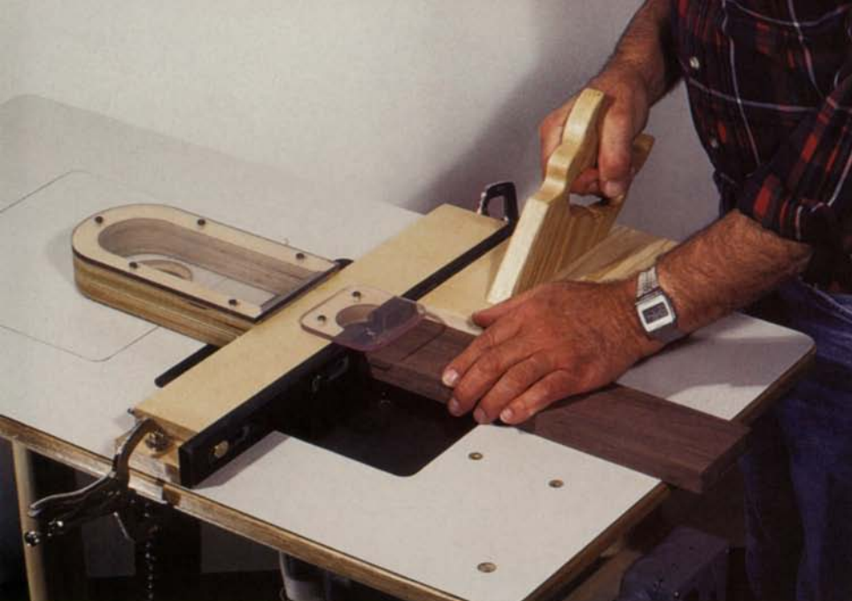
The router jig above is used to trim templates that are the same width as the distance between the router's edge and the cutting edge of the bit.
