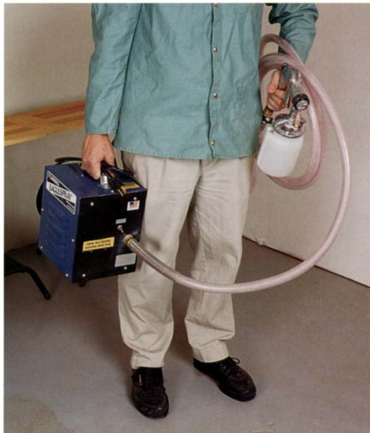
Portability is one of HVLP systems' greatest advantages. Most small, single-stage turbines, like the EagleSpray Turbo shown here, are light and have a handle so that the unit, its hose and the spray gun are easy to carry.
