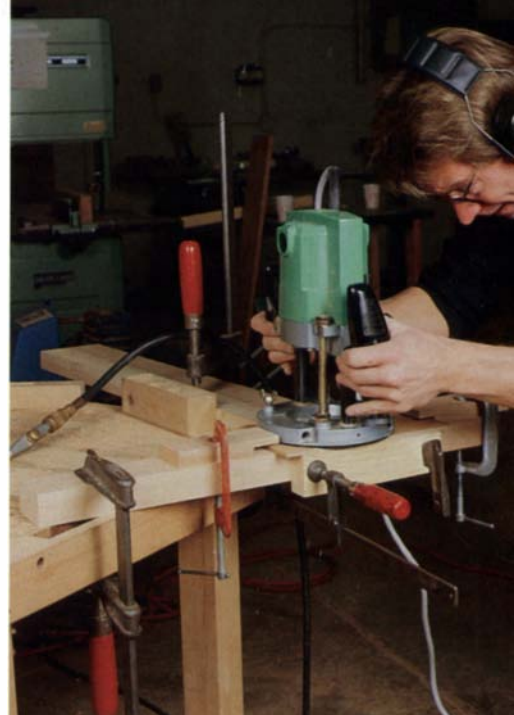
A plunge router and a simple L-shaped guide clamped to the leg are used to cut mortises in the legs. Here, the side rail is inserted into its mortise in the leg, and the author is routing through the leg and the side-rail tenon to form the interlocking rail-to-leg joint. The notched wood blocks flanking the template are stops for setting mortise length.
