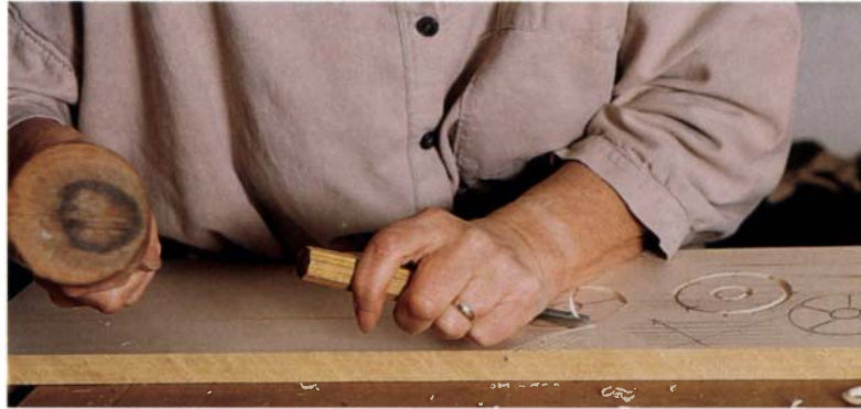
The first step in carving a flower is to outline the shape with a V-shaped parting tool. Carving the outline, as opposed to scoring it with vertical cuts, removes wood and gives you space to work.
