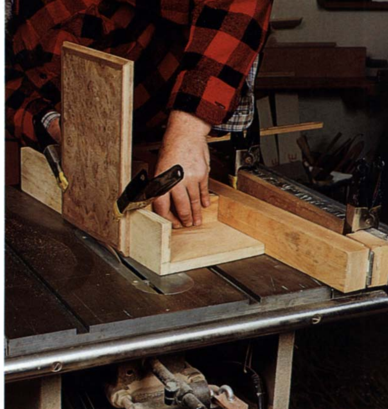
The edge of the box lid is coved on the tablesaw. Numerous shallow passes are made over the blade guided by a rip fence, the angle of which determines the shape of the cove cut. Cummins uses a simple jig to support the workpiece and to shield his hands from the blade.
