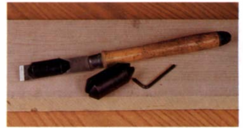
Taming of the skew is accomplished with Stabilax, an attachment that provides easier and safer results with this difficult-to-use tool.
