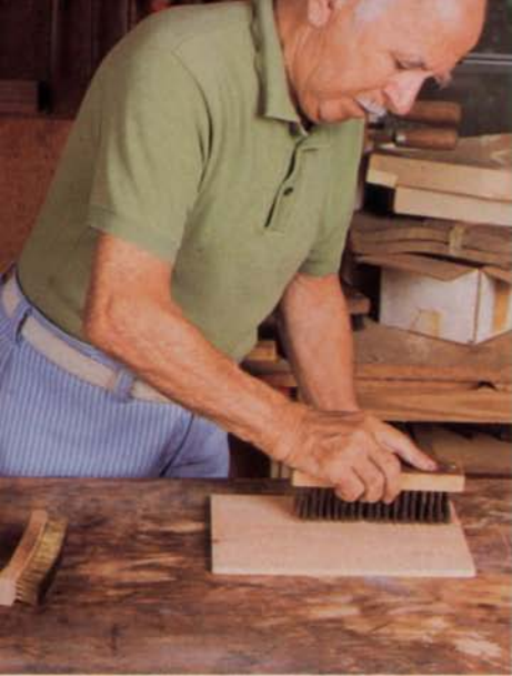
Left: To clean the wood's pores of impurities before filling, Frank uses a soft-steel-bristle brush, scrubbing lightly and with the grain. The brass-bristle brush on the bench can also be used. Right: After
