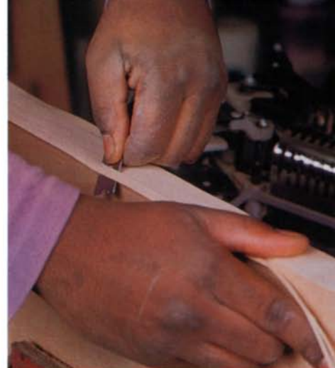
Left: It's simple to apply preglued edgebanding tape with a hot iron that melts the glue. Keep the iron moving and press the tape down with the rounded edge of a piece of wood. Above: After ironing on the tape, it is trimmed with a single-edge razor blade and the corners are lightly sanded.
