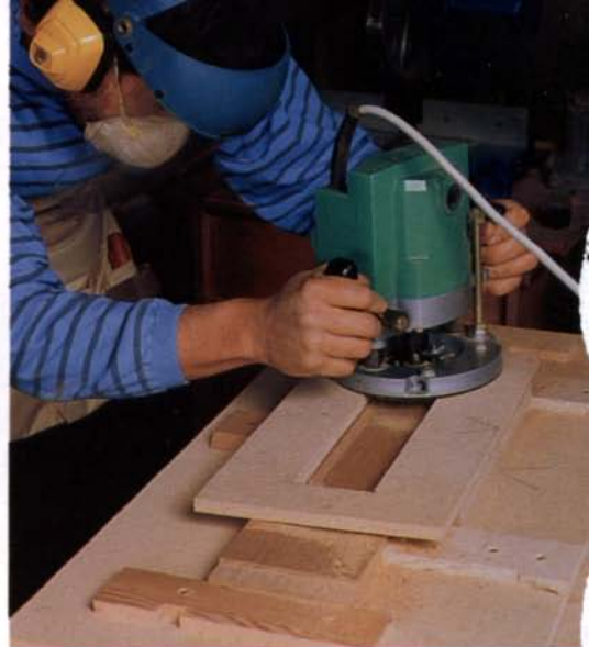
cut out the drawer opening in the front apron, the author uses a plunge router fitted with a guide bushing that follows a rectangular hole cut into a particleboard template. With the template clamped on top of the apron, he plunges the bit and follows around the template clockwise, cleaning up the corners of the opening with a chisel after routing.
