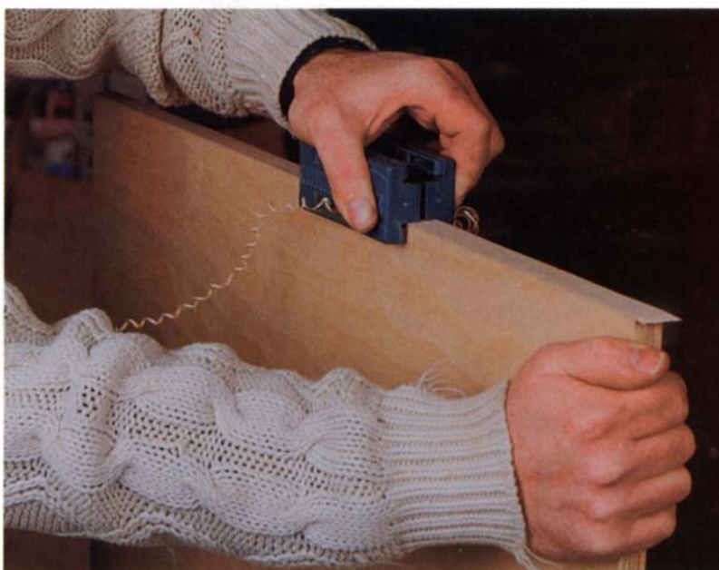
The Virutex edgebander comes with this trimming tool that cuts both sides of the tape at the same time.
