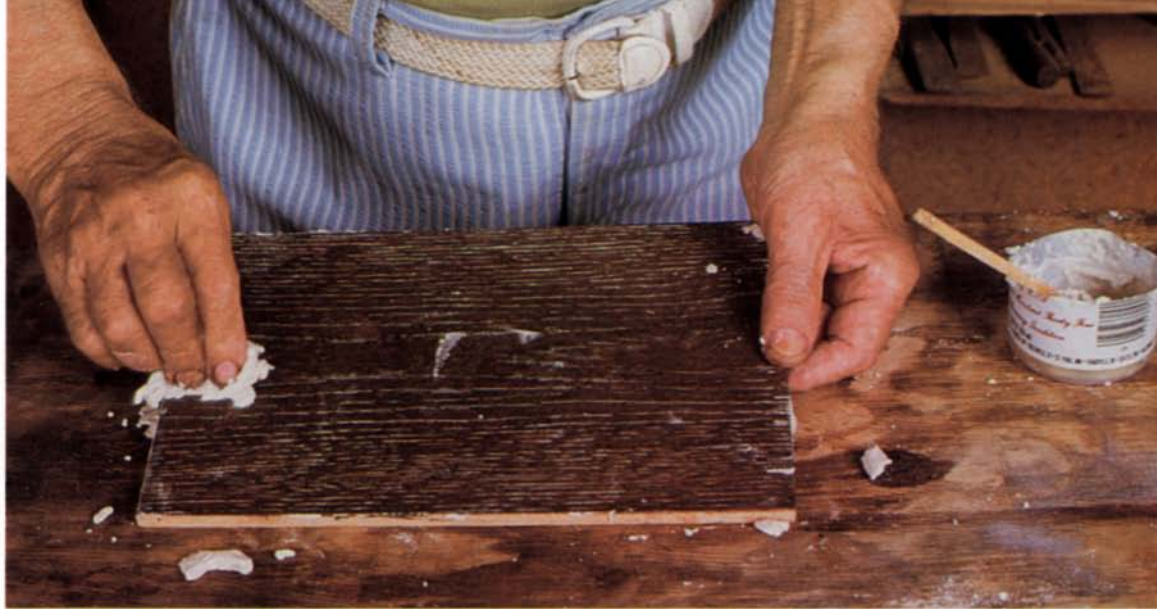
Left: To clean the wood's pores of impurities before filling, Frank uses a soft-steel-bristle brush, scrubbing lightly and with the grain. The brass-bristle brush on the bench can also be used. Right: After
