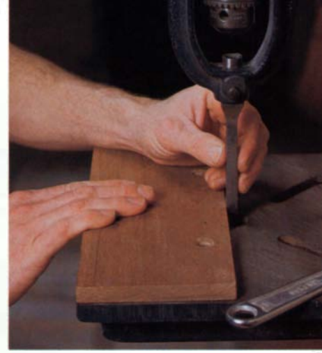
Above: After the chisel holder and chuck are installed, the chisel is inserted in the holder and advanced until it extends through the table's center hole. Then the chisel's front face is aligned parallel to the front edge of the table. Left: As the author uses a hollow-chisel mortising attachment on his drill press, a dust collector vacuums up debris. The stop block clamped to the auxiliary fence positions the workpiece so he can cut one end of a mortise.
