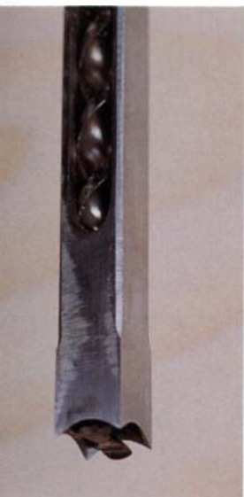
Left: The auger has been inserted up through the hollow chisel, with about 1/32-in. clearance between its cutting edges and the chisel's beveled edges (to prevent wear), and its shank has been secured in the chuck. The author has ground the corners of this chisel to reduce friction when mortising. Right: Erickson adjusts the fence to center the chisel between lines on a test piece and cuts a practice mortise. Debris is expelled through the chip-ejection slot and a hold-down clamp retains the workpiece in order to withdraw the chisel.
