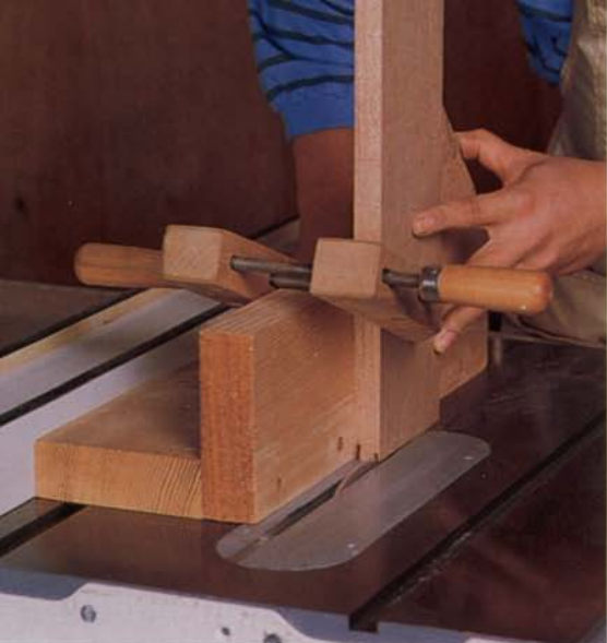
Left: To cut the male dovetails on the ends of the side aprons, Kapuaala uses his tablesaw and homemade tenon jig, which supports the workpiece vertically as it is guided past the tilted blade. Center: After crosscutting the female sliding dovetails in the front and rear aprons with a miter gauge on the tablesaw, Kapuaala pares the bottom of each flat with a chisel. Right: To
