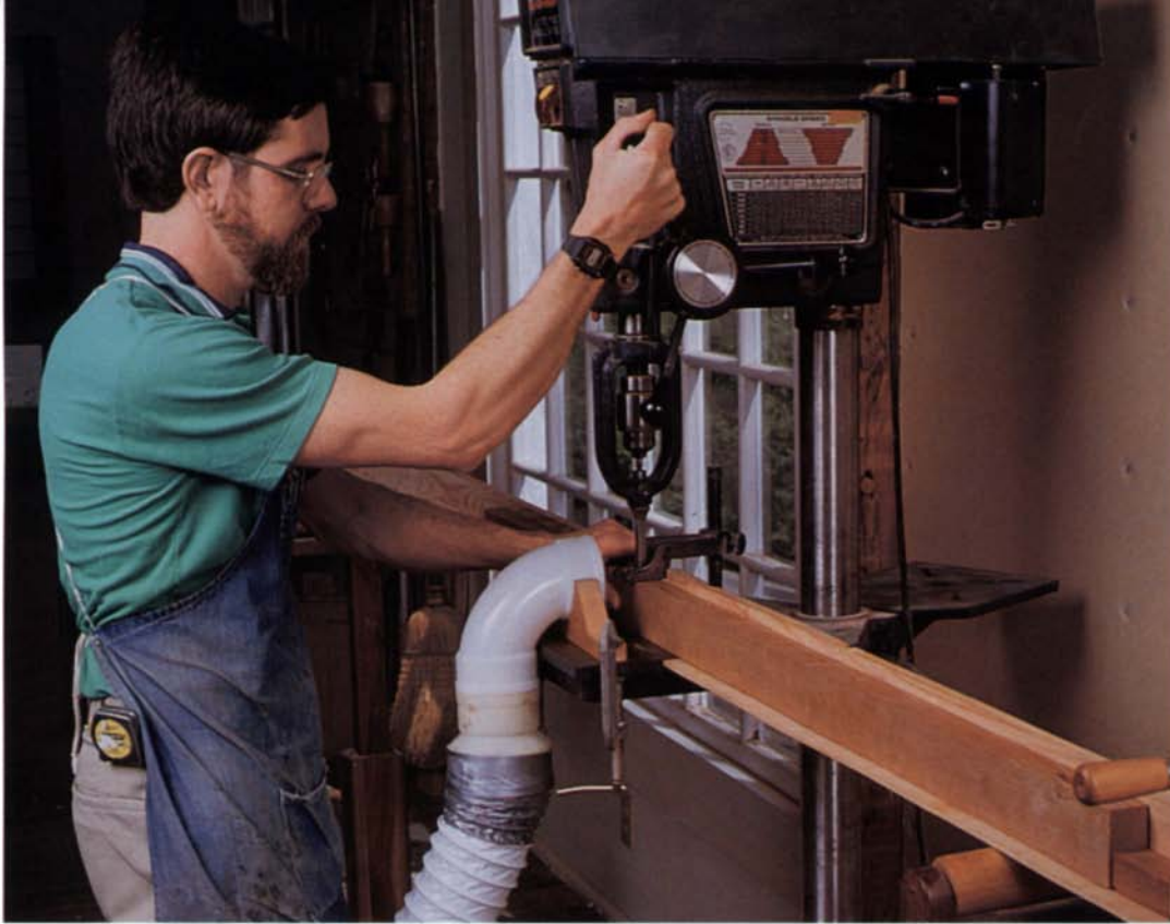
Above: After the chisel holder and chuck are installed, the chisel is inserted in the holder and advanced until it extends through the table's center hole. Then the chisel's front face is aligned parallel to the front edge of the table. Left: As the author uses a hollow-chisel mortising attachment on his drill press, a dust collector vacuums up debris. The stop block clamped to the auxiliary fence positions the workpiece so he can cut one end of a mortise.
