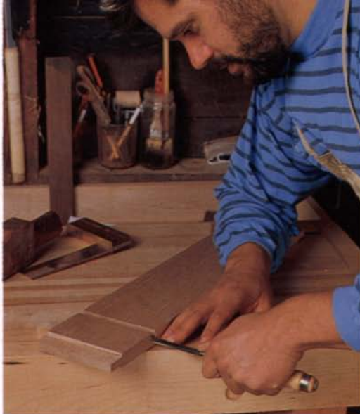
Left: To cut the male dovetails on the ends of the side aprons, Kapuaala uses his tablesaw and homemade tenon jig, which supports the workpiece vertically as it is guided past the tilted blade. Center: After crosscutting the female sliding dovetails in the front and rear aprons with a miter gauge on the tablesaw, Kapuaala pares the bottom of each flat with a chisel. Right: To
