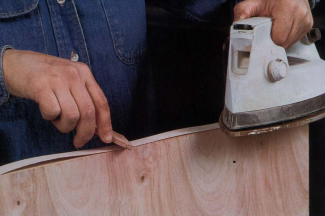
Left: It's simple to apply preglued edgebanding tape with a hot iron that melts the glue. Keep the iron moving and press the tape down with the rounded edge of a piece of wood. Above: After ironing on the tape, it is trimmed with a single-edge razor blade and the corners are lightly sanded.
