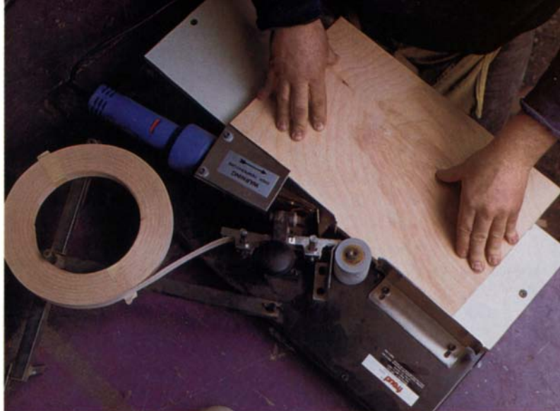
The Freud edgebander can apply preglued tape to panels up to 2 ft. wide by 3 ft. long without table extensions. It melts the tape's glue, automatically applies the tape and has a cutter to trim the tape to length. It sells for about $300.
