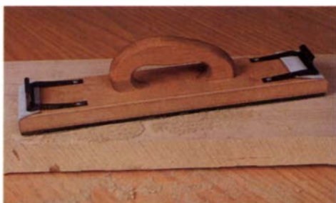
A plate-glass bottom on the Donnell sanding plane provides a flat surface for fine finish-sanding.
