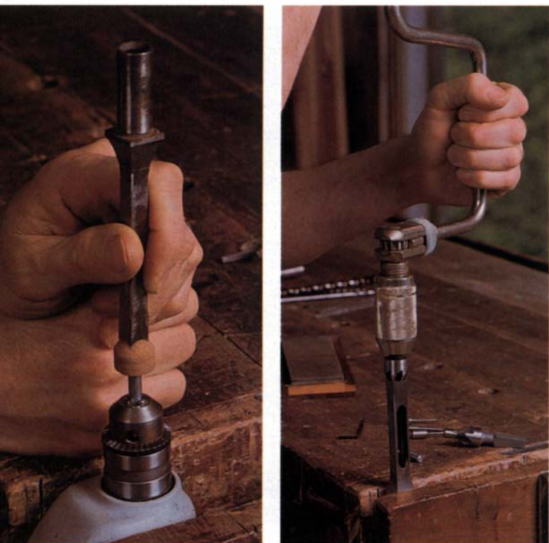
Left: The author grinds the inside bevels of a hollow chisel by lowering its end onto a conical-shape stone turning at about 1,000 RPM in a hand drill. Edges are ground only until sharp, and burrs are removed by honing the chisel's outside on a flat stone. Right: Erickson prefers to sharpen hollow chisels by grinding their bevels with high-speed-steel, countersink-like bits turned by hand. The bits have fixed or interchangeable pilots that center them in the chisel.
