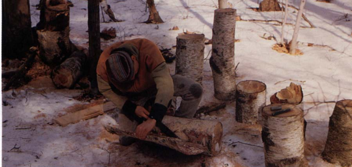
The author peels birch bark from the log with a 2-in. slick. The board lying behind him can be used to help hold the bark out of the way as the work progresses.
