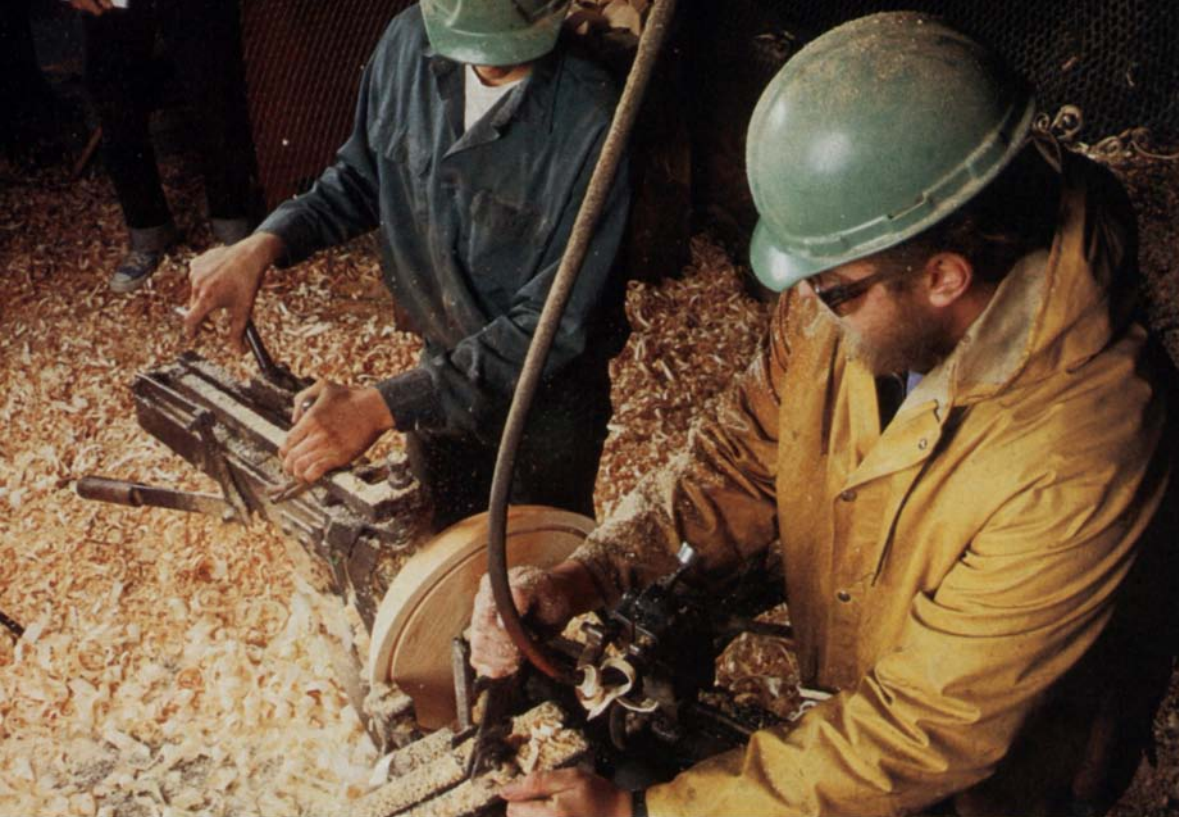
Left: With a backband knife, a worker removes the stub that remains after turning the outside of a bowl, while Boudwell begins the next cut that will form the inside of one bowl and the outside of the next smaller bowl. Above: the curved arm and tip of the cutting knife determine a bowl's size. The rectangular back plate that locks the arm to the lathe is hidden behind the blank.
