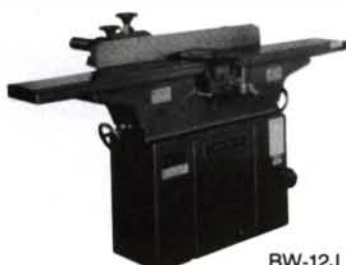
JOINTER $2,495. Planes 12" wide and up to 1/2" deep. Four knife cutter head. 3 HP US motor. Other models from 6" to 16" wide.
