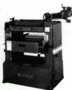
BW-612PVG PLANER $6,195. Planes 24" wide by 9" thick. Top & bottom rolls drive 10 HP US Main Motor. Other models from 12" to 24" wide.
