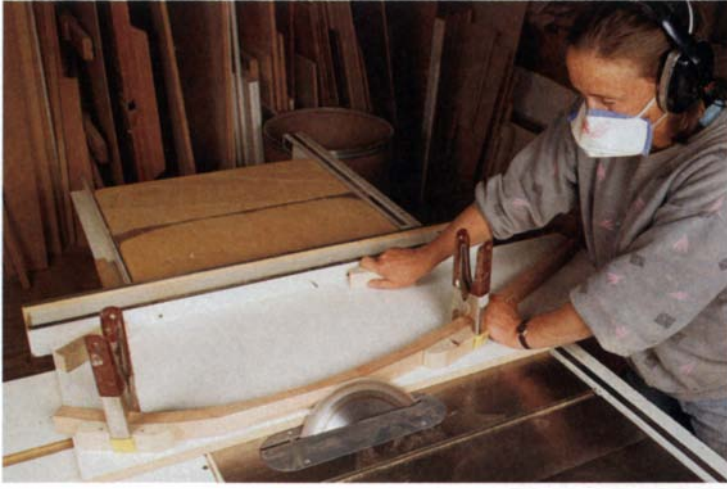
The facets for joining the legs are cut on the tablesaw by clamping the legs one by one to a jig. Position the leg on the jig by aligning the joint's centerline, which is transferred from the laminating form to each leg, with a corresponding line on the jig. The jig is reversed and the leg is clamped to the blocks on the opposite edge to cut the adjacent facet.
