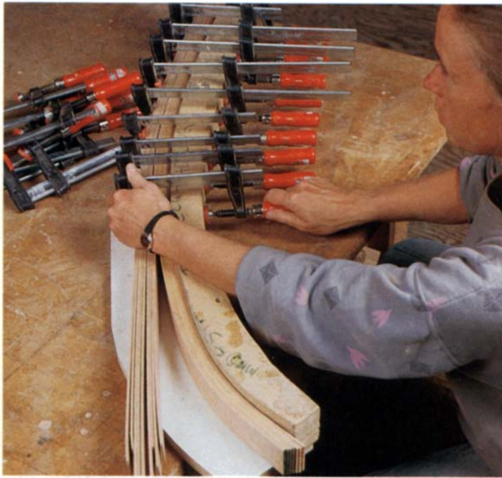
After eight hours the clamps are removed from one of the laminated legs. Note the unglued laminations that Ames uses as cauls to clamp the glued-up laminations to the form.
