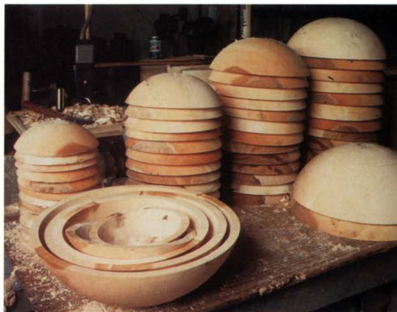
The bowl lathe at Granville can turn as many as seven bowls from a single block of wood in as little as six minutes. The nested bowls in the foreground were all cut from the same block of birch.
