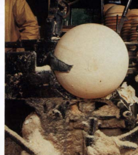
Left: With a backband knife, a worker removes the stub that remains after turning the outside of a bowl, while Boudwell begins the next cut that will form the inside of one bowl and the outside of the next smaller bowl. Above: the curved arm and tip of the cutting knife determine a bowl's size. The rectangular back plate that locks the arm to the lathe is hidden behind the blank.
