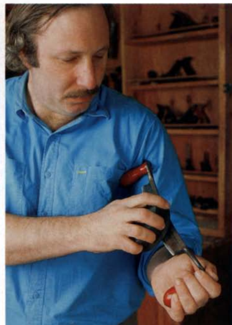
Left: A large, straight-blade drawknife is tops for quickly hogging away large amounts of stock, especially in green wood. With a workpiece secure in the shaving horse, the author twists the knife as he pulls it through the cut, using leverage to split off the waste. Above: Holding the drawknife in his arms like a fiddle, Starr uses a round axe-sharpening stone to touch up the edge.
