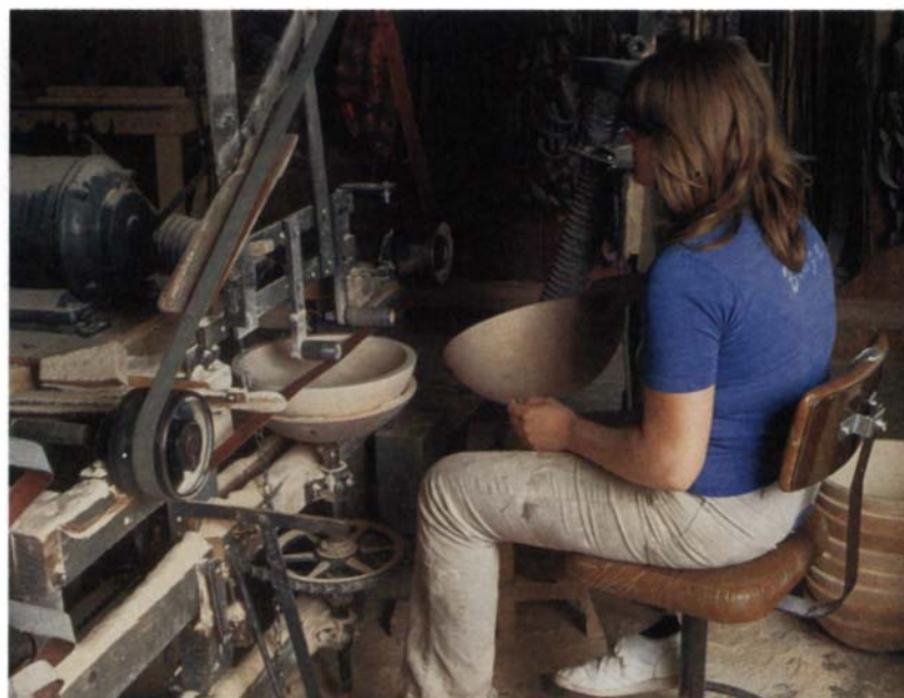
The rough tool marks left by the lathe are removed in a series of sanding operations. A worker places bowls on a revolving table, which automatically belt sands the edge of each bowl.
