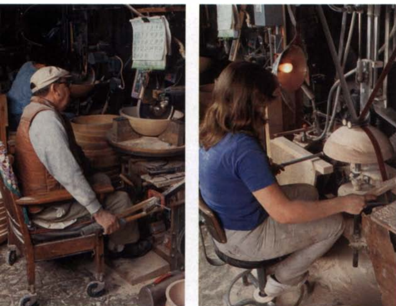
The operators control the pressure of the belt sanders with various levers and pedals as they sand the inside (above left) and outside (above right) of each bowl.
