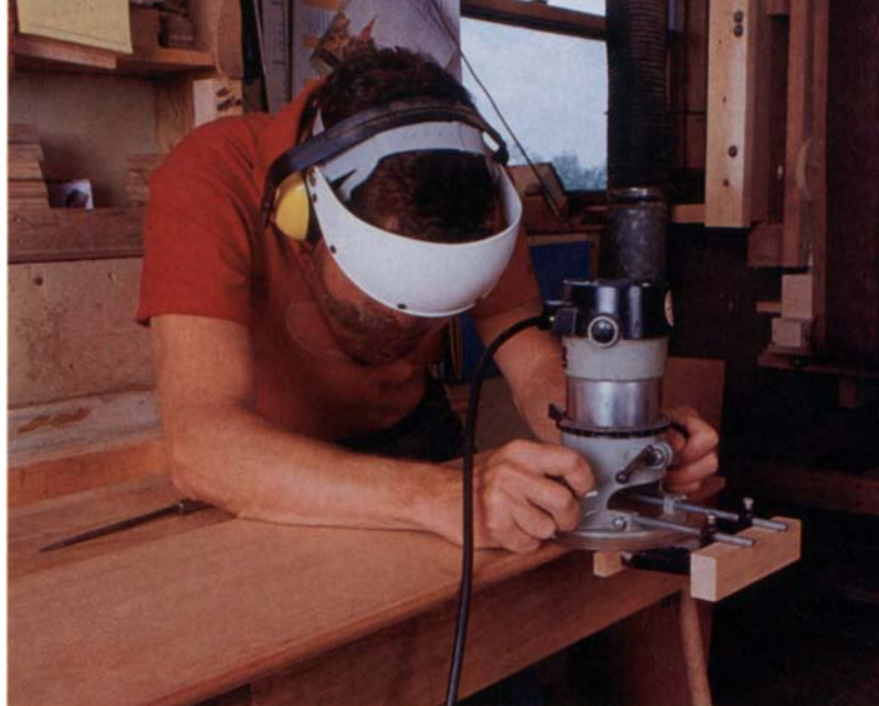
To ensure proper hinge placement, Campbell uses a fence when routing the hinge mortises.
