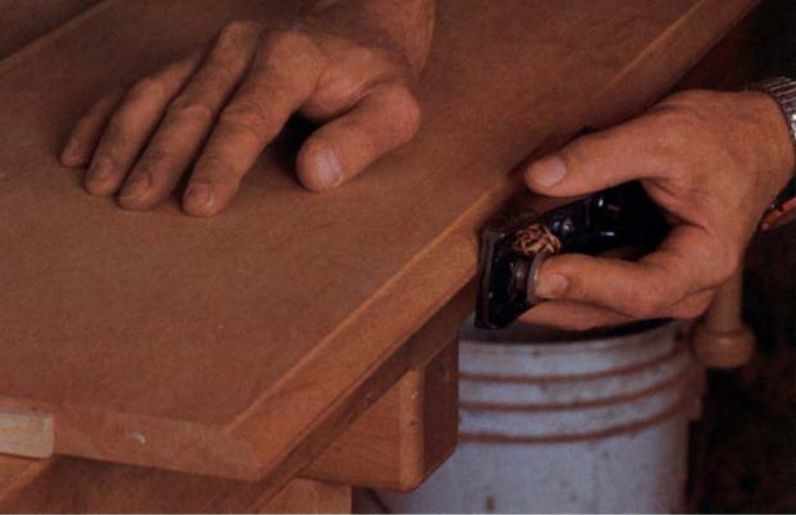
A few passes with a block plane are required to round over the flat portion of the table's edge left uncut by the roundover bit.
