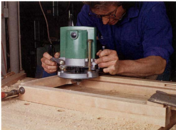
With the side frame clamped to the workbench, Rogowski routs the panel groove with a bearing-guided slotting bit. A 1/2-in.-thick board is laid atop the shaped rail to fill the setback between the inside surfaces of the rail and leg, providing a consistent surface for the router base.
