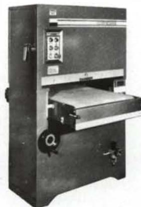
BWS-25 WIDE BELT SANDER $6195. Sands stock 25" wide by 5 7/8" thick. 10 HP 3 phase main motor. Fixed Feed Rate of 15"/minute. Other models from 13" to 37" wide, fixed and variable feed rates.
