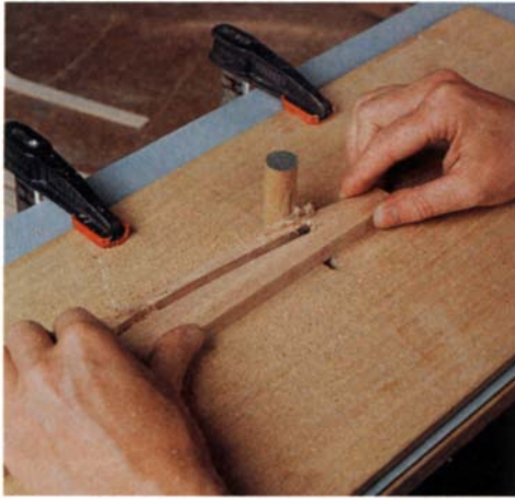
With a shopmade single-point guide fixture clamped to the router table, Ames routs the adjusting slot parallel with the back curve of the vertical support.
