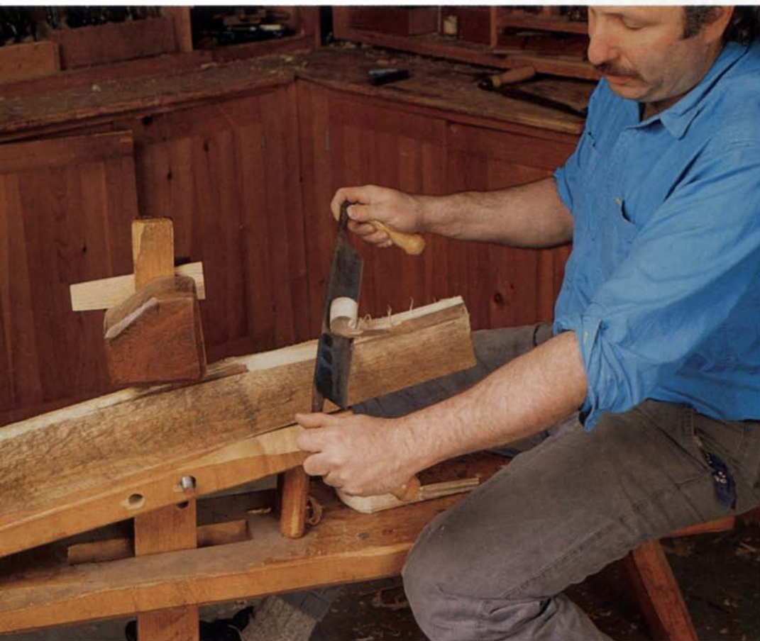
Left: A large, straight-blade drawknife is tops for quickly hogging away large amounts of stock, especially in green wood. With a workpiece secure in the shaving horse, the author twists the knife as he pulls it through the cut, using leverage to split off the waste. Above: Holding the drawknife in his arms like a fiddle, Starr uses a round axe-sharpening stone to touch up the edge.
