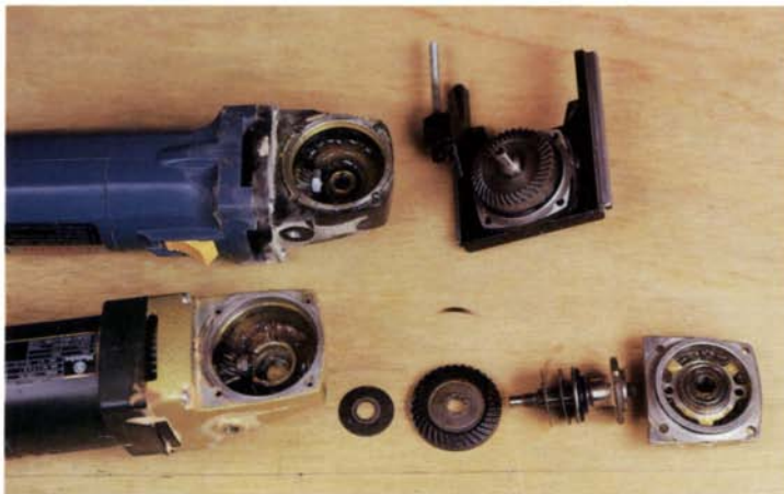
Although externally similar to the Freud machine, the Lamello's power train (bottom of photo) is protected against impact loading by a spring clutch. Freud's ring gear (top of photo) is unyieldingly pressed to the cutter shaft.
