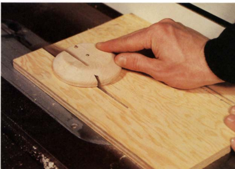
A piece of plywood serves as a carrier for ripping crescents from the shaped discs. The discs are fastened to the plywood with two ⅛-in. brazing rod pins. Set the fence as shown, above, to cut the desired crescent size. After ripping off one crescent, rotate the remaining piece 180° and rip off the second.
