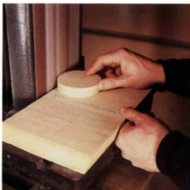
Each disc is rotated on a pin and trued against a sanding belt, above left. Two pins secure the disc when its back edges are routed, above right. Plexiglas shims under the disc provide clearance for the chamfer bit's bearing guide.
