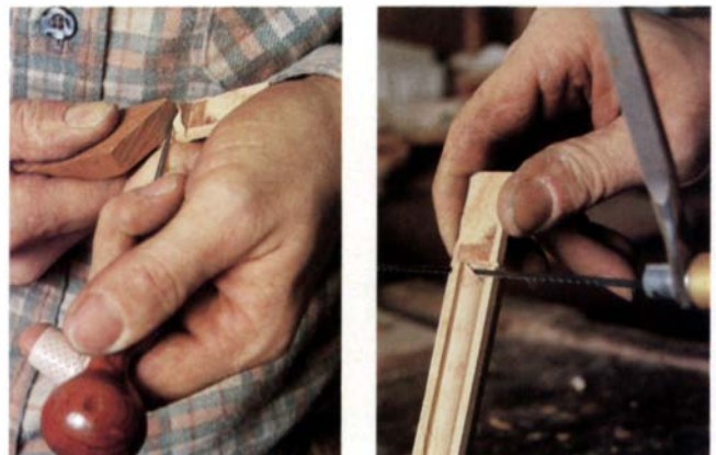
The first step in hand coping a joint is to scribe the cope line with a 45° marking block (left). The second step is to saw to the line with a coping saw (right).
