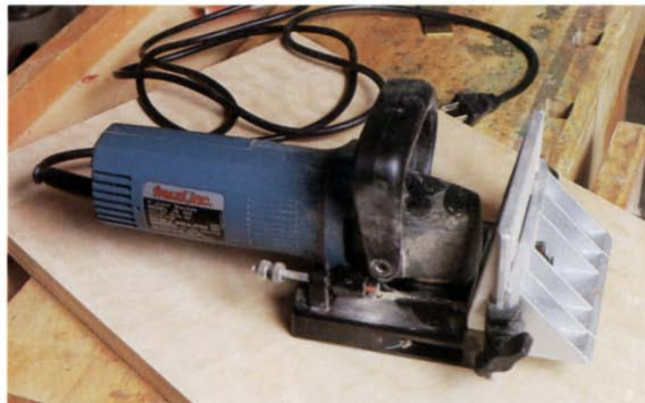
Freud's made-in-Spain model JS100, above, makes plate joinery affordable for the amateur and small-shop professional woodworker. To plate-join miters, the fixed-angle front fence, adjustable via wing nuts on either side, is removed and reversed.
