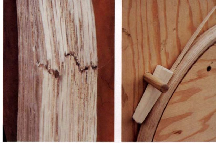
Examples of bending failures due to brash failure (left) and excess tension (right) illustrate what can go wrong when wood fibers don't cooperate with your bending efforts.
