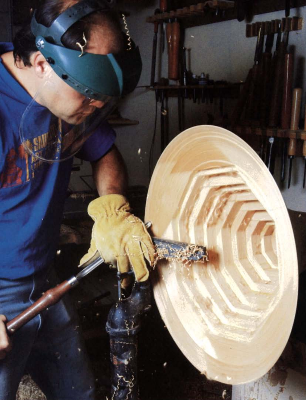
Sterba uses the shoulder of a deep-fluted gouge to shear the ridges from the lamination, left, and to shape the inside of the bowl. The bowl bottom is carefully finished with light scraper cuts, above.
