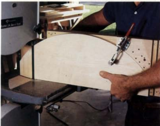
Tapering jig does double duty: author uses jig on edge to rough-cut taper on the bandsaw, then repositions fence and flips jig over.
