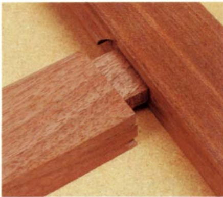
Rails and stiles meet with just a short cope; face of mortise is chiseled square.
