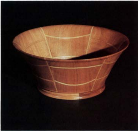
The author glues up bowls from staves tapered on the tablesaw. Angled blocks set the miter gauge and blade angle.
