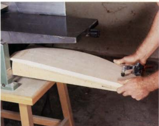
Jig passes through the planer for final trimming. Be sure to shut off the planer and pull the jig through after it stops feeding forward.
