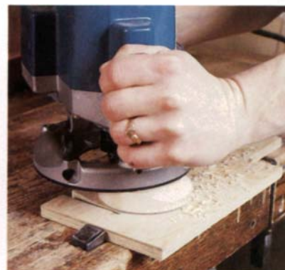
Each disc is rotated on a pin and trued against a sanding belt, above left. Two pins secure the disc when its back edges are routed, above right. Plexiglas shims under the disc provide clearance for the chamfer bit's bearing guide.
