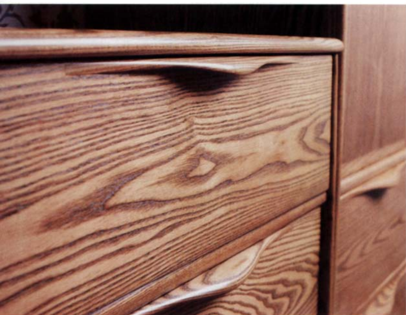
Handshaped hardwood pull adds a distinctive touch to drawers. The pulls are coved on a tablesaw, then shaped on a bandsaw.
