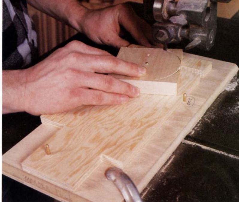
Discs are cut from 3¼-in. squares on a jig mounted to a bandsaw table. A hole is bored in the center of each square, so it can be mounted on a swinging arm, which carries the blank into the blade as it's rotated through the cut. The pin on the arm is located so that the distance between it and the blade equals the radius of the disc and is tangential to the blade's line of cut. A stop pin secures the arm in cutting position.
