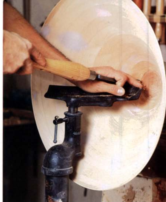
Sterba uses the shoulder of a deep-fluted gouge to shear the ridges from the lamination, left, and to shape the inside of the bowl. The bowl bottom is carefully finished with light scraper cuts, above.
