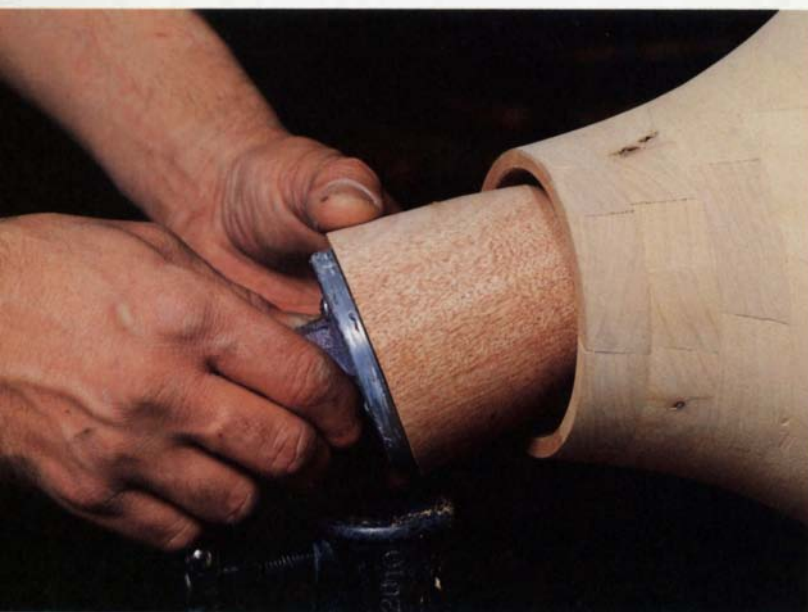
A faceplate screwed to a 3-in.-long tapered plug is glued into the bottom of the turning before the bowl is finish-turned.
