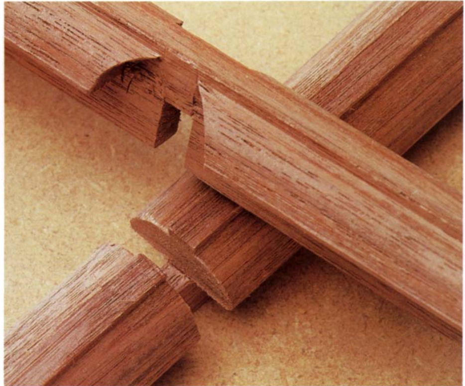
You don't need matching cope-and-stick bits to make this overlapping scribed joint. More complicated shapes, such as those shown below, can be coped similarly, with just a few more straight chisel cuts to fit the outside edges.
