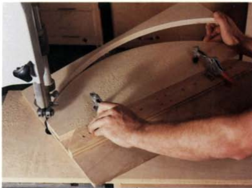
With work held securely by quick-action clamps, Tinius' radius jig bandsaws curves for the top slats quickly and accurately.
