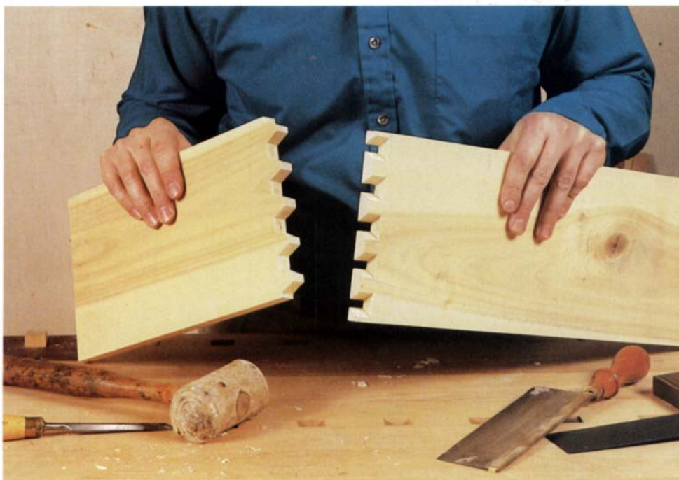
Trimming waste on the wrong side of the layout line can lead to some strange dovetails.
