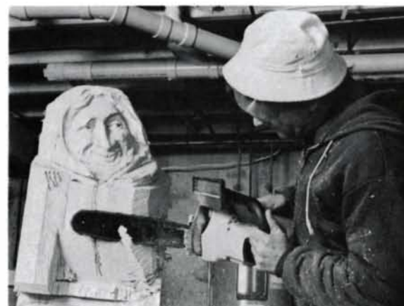
A chainsaw wastes most of the figure, and is also used as a power rasp.
