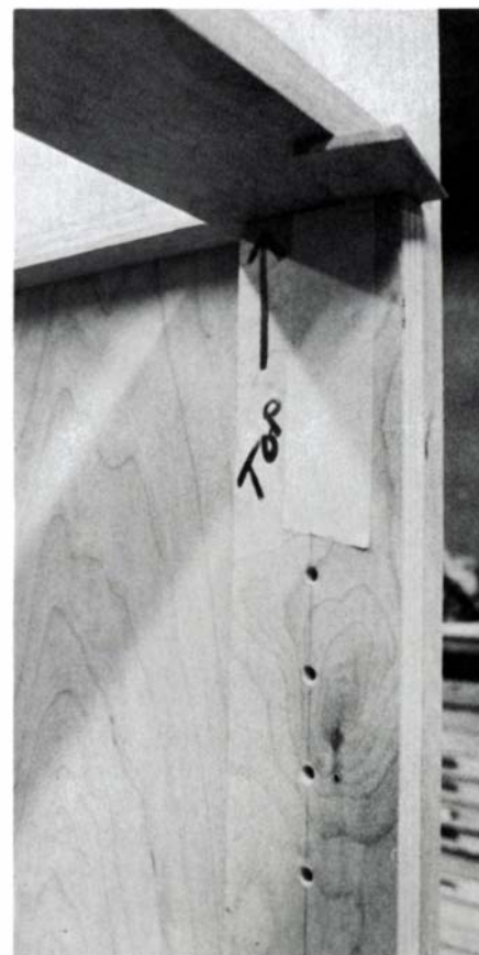
A plywood template, wedged inside assembled carcasses, speeds boring of shelf-pin holes, which should be spaced about 1\frac{1}{2} in. apart.
