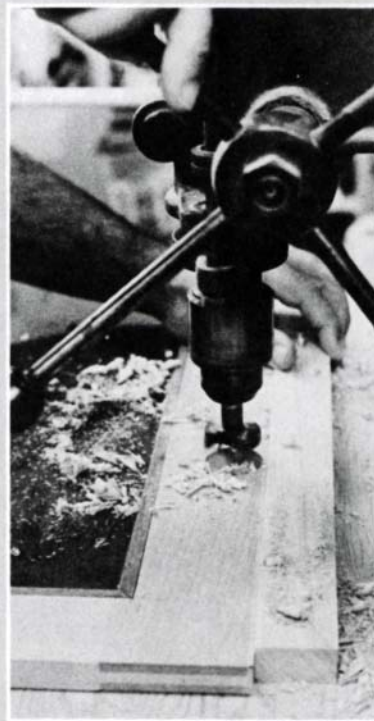
Most European-style concealed hinges have two parts—a baseplate that attaches to the inside of the carcass, and an arm-on-flange that fits into a round mortise in the door. The top hinge opens about 100°; the lower, 176°. Made by Grass, both self-close, and are available for either inset or overlay doors. The bit bores a 35mm round mortise.
