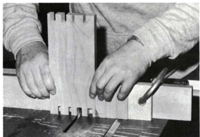
Once marked out, the pins are formed by wasting the wood between with dado-blade cuts. In the photo below, Duginske completes the second series of pin cuts.
