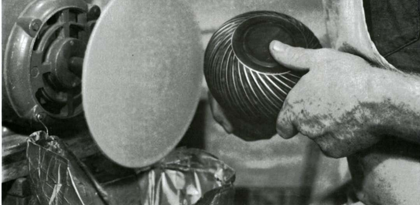
After the grooves are cut on the plywood sanding disc, Hunter uses a foam-backed disc to refine the shapes.
