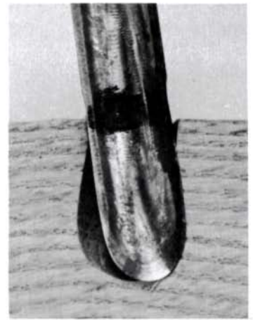
The spoon bit at top is as it comes from the manufacturer. The one below it has been modified into a duckbill for boring the chairmakers' mortise, shown at right. When shaping the bit, maintain full diameter just behind the cutting lip, but relieve the sides so that the bit can pivot in the hole to enlarge the bottom without enlarging the opening. The mark on the bit is a depth gauge.
