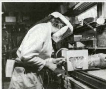
Dust-free and breezy inside his 3M Airhat, Hunter turns a bowl in the dust-collection box drawn below.
