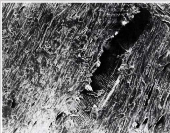
These scanning electron microscope photos illustrate why a crisply cut surface is better for gluing than a handsawn one. The photo of hand-planed maple at left shows cleanly sheared fibers
