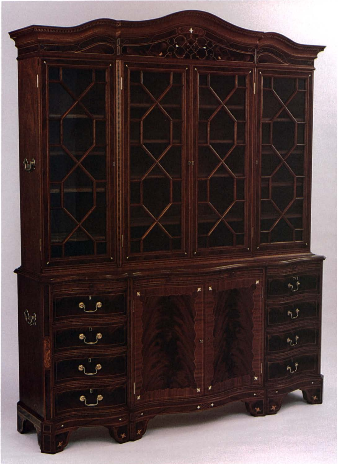
Adapted from an original built in Charleston, S.C., around 1790, Heisey's Hepplewhite breakfront is made of solid mahogany. The serpentine doors are coopered, the drawer fronts sawn from 3-in. thick boards. Both are veneered with crotch mahogany.
