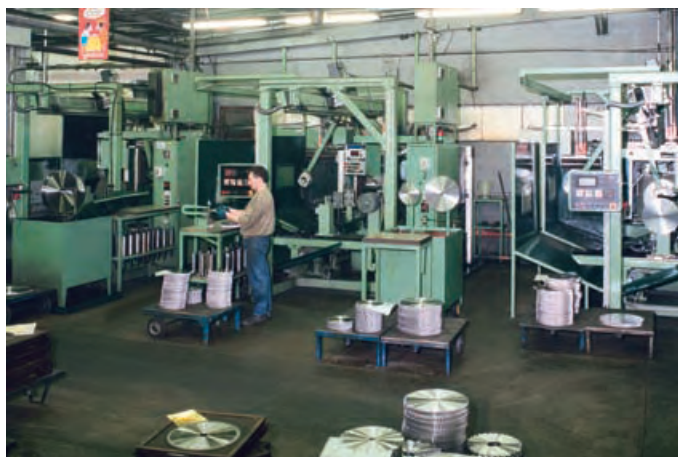
Grinding and tensioning the blades.
