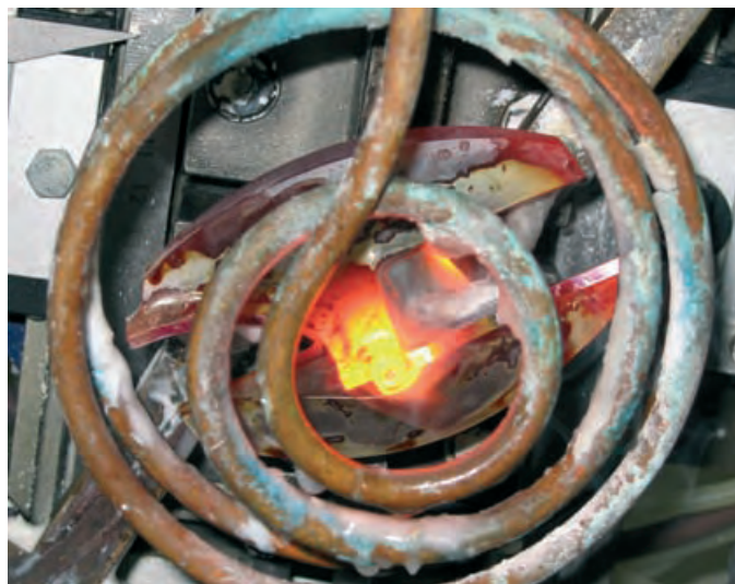
680°C in seconds - and the brazing is complete.
