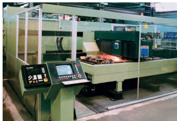
Laser cutting the steel plates.
